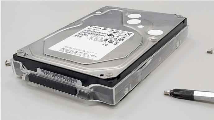
2. Pull the disk carrier up and off the HDD, be careful not to twist the carrier.
