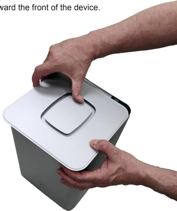
2. Lift the cover to expose the hard disk drives.
