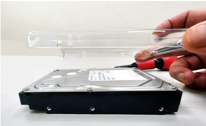
3. Replace the problem HDD with a new HDD of the same type. Follow steps 1 and 2 above in reverse order to install the new HDD. Make sure the carrier is oriented so the handle is located at the 'top' of the HDD when inserted into the enclosure. The 'bottom' of the HDD includes the SATA interface and power connection that will be seated in the SATA port. The correctly positioned carrier allows free contact for the SATA and power connections.
