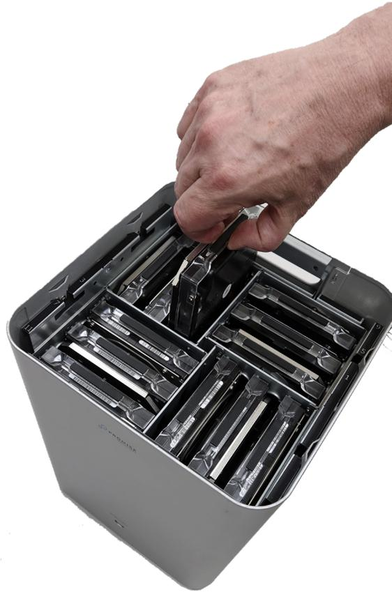
4. To replace the new hard disk drive and disk carrier assembly, insert the drive and carrier oriented in the same way when it was removed. Slide it in until it is firmly seated. The drive remains in place without any additional hardware mechanism such as a latch. It fits snugly in place to remain securely seated.
