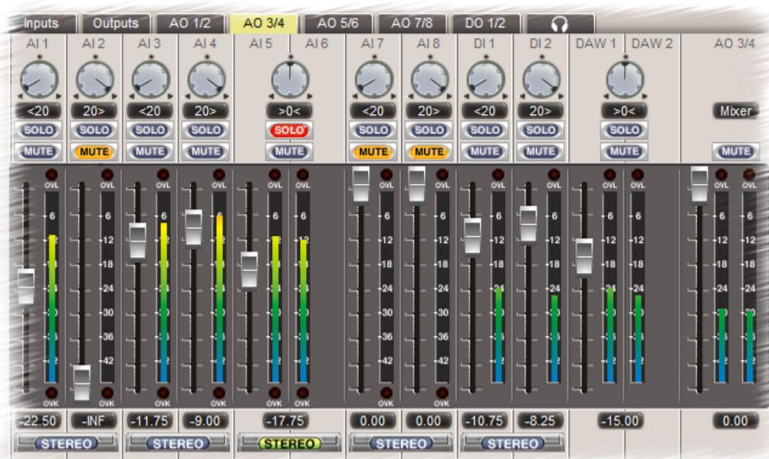
Each input has a fader, a high-resolution [peak meter](#), with overload indication 0.05dB below clipping, plus mute and solo buttons and a pan-pot. By engaging the 'Stereo' button beneath an input pair, the pair is controlled by a single stereo fader, mute button and solo button, and the pan-pots are replaced by a single balance control. The DAW contribution and output strip are always in stereo mode.
