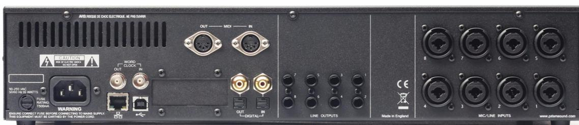
Atlas's rear panel contains all Atlas's connections, except for the instrument inputs and headphone output, which are on the [front panel](#).
