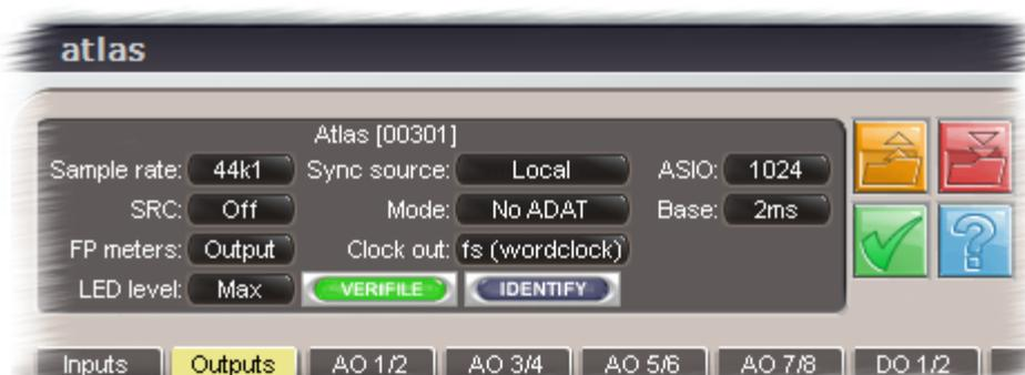
The Atlas model and serial number are displayed at the top of the Unit settings area. Note that the currently-installed firmware version of the Atlas unit can be displayed by hovering the mouse cursor over this text.
