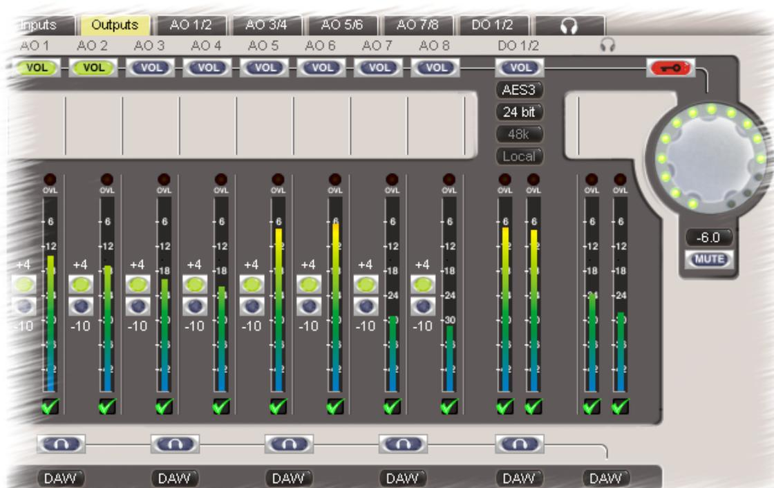
Line output level is switched between +4dBu and -10dBV nominal by the '+4/-10' radio buttons.
