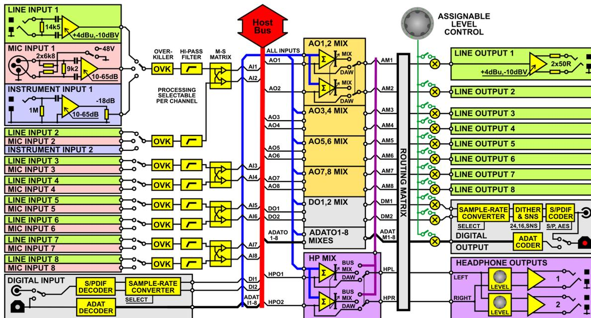
The figure above is a simplified block diagram of the Atlas audio signal paths.
