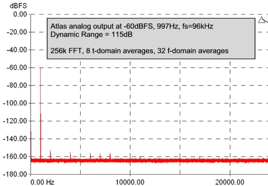
Except where otherwise stated, audio performance data are typical, RMS, unweighted, 20Hz..20kHz figures, measured at 997Hz, using fs=96kHz and '+4dBu' sensitivity settings.
