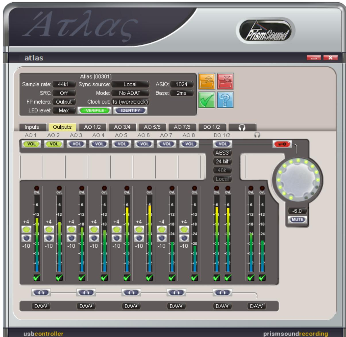
Whilst Atlas can be controlled in a limited way from within the Mac or Windows operating system, or by some audio application programs, most of its detailed features can only be accessed using the Atlas Control Panel app.
