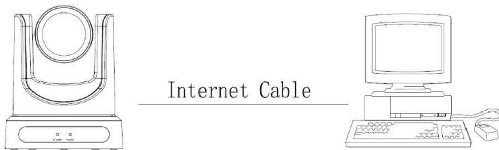
**Picture 1.1 Direct connections via “cross-over” network cable**
