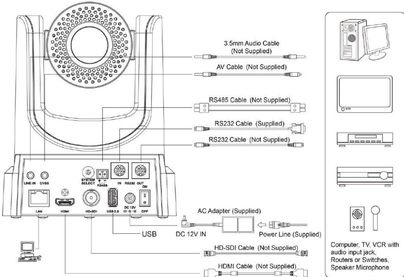
**Step2.** Set the system select switch for your desired video output resolution and frame rate.
