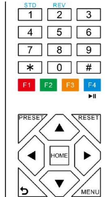
1. To store a preset position: The user should manually setup the desired shot using the Pan Tilt and Zoom controls. Press the [PRESET] button first and then press the numeric button [0-9] to which you want to assign the shot. Ten total preset positions (0-9) are available from the IR remote control (255 available via RS232/RS485/IP Interfaces).
