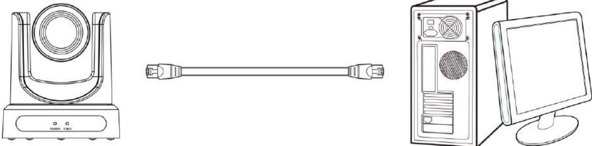
**Picture 1.1 Direct connections via “cross-over” network cable**
