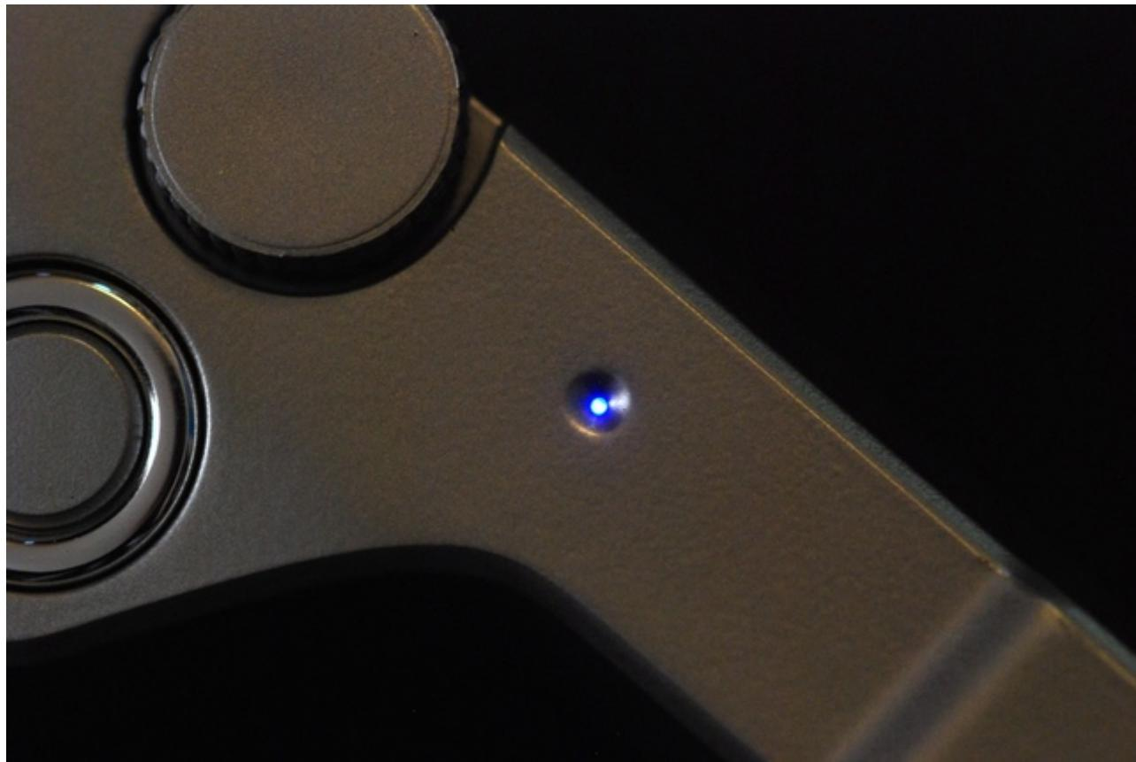
The blue battery indicator light on Pictar comes on when any of the dials are activated and pulses gently to show the battery is in a good condition. The light stops flashing after 45 seconds of inactivity.
