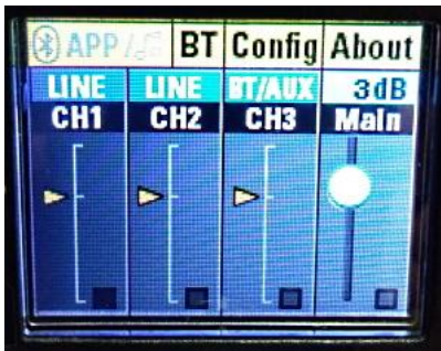
Fig. 3 Main (Master) Channel Gain +3 dB
