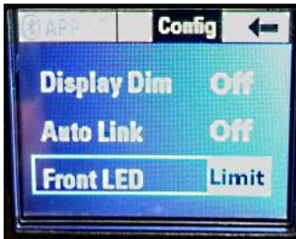
Fig. 55 Front LED parameter set to Limit
