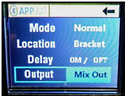
Fig. 30 Output Parameter, Mix Out Selected
