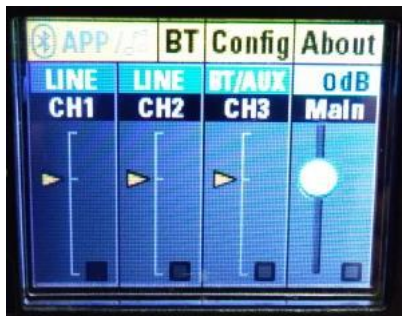
Fig. 2 Main (Master) Channel Gain (Default)
