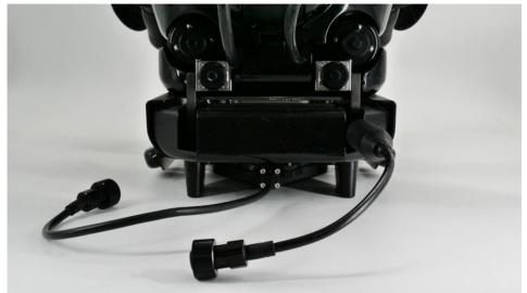
1.6.2. Please attach the connector of the Q-DVL to the A3 or A4 Q-interface only. Attach the connector of the side scan sonar to any Q-interface on the ROV.
