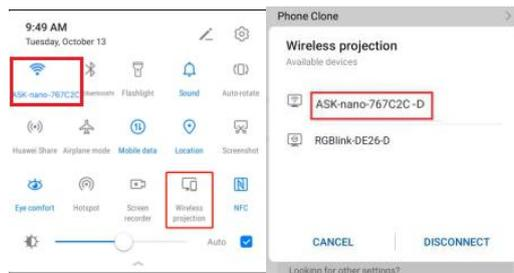
**Tip:** When clicking "Wireless Projection", select "Yes" on WLAN setting, and the mobile phone does not need to be connected to any LAN WIFI.
