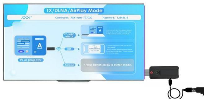
**Tip:** Power to RX is essential, please prepare a power supply port or power adapter before RX installing. If the display offer USB power port, use it to supply power for ASK nano RX.
