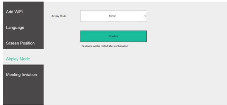
" Mirror" means to cast the current image of the iOS device, while "streaming" means that when using iQIYI, Tencent and other video APPs on iOS device to play video, the video is only played on big screen instead of on Below is an example when AirPlay is set as Streaming, the iQIYI video page on iOS device:
