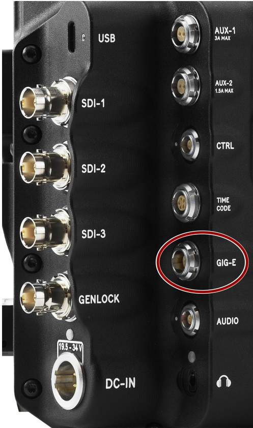
Figure: Front Face of the GIG-E Connector (looking at the back of the camera).
