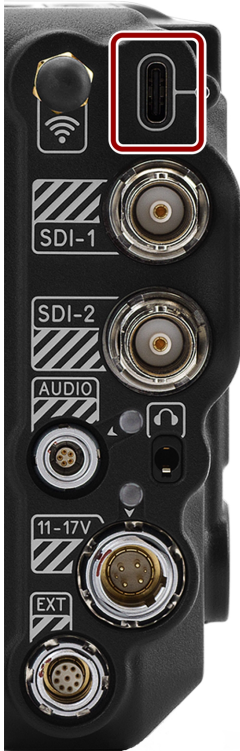
Figure: Front face of the USB-C port (looking at the back of the camera).
