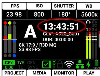
**NOTE:** The timecode is reset when the camera is turned off.
