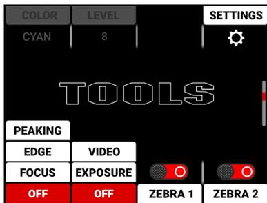
The LCD Tools page is the third page on the LCD. Press the down button twice to navigate from the Home page to the Tools page.
