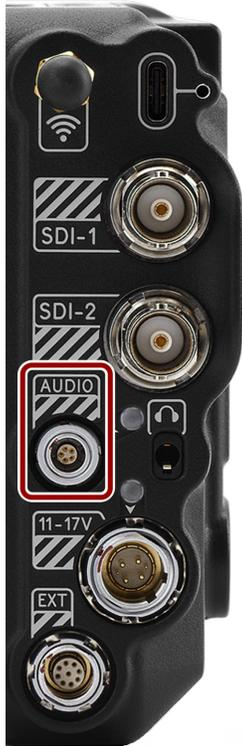
The female 5-pin 00B audio connector accepts 2-channel audio, Line, Mic, and +48V Phantom Power.
