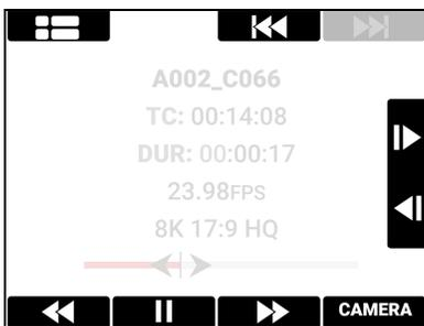
With the Playback screen buttons you can view the Clip list, move to the start of the clip, fast reverse, play/pause, fast forward, and move forward and reverse by a single frame.
