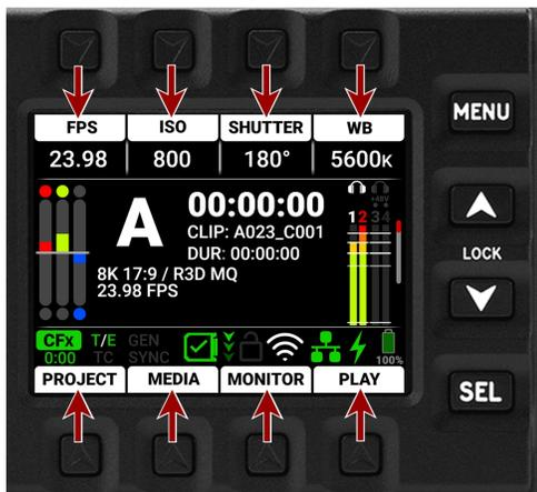
In this example, pressing the button above FPS opens the Recording Frame Rate selection list:
