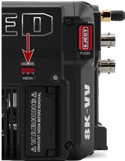
3. Press the CFexpress media card until the lock release clicks. The card will spring out slightly.
