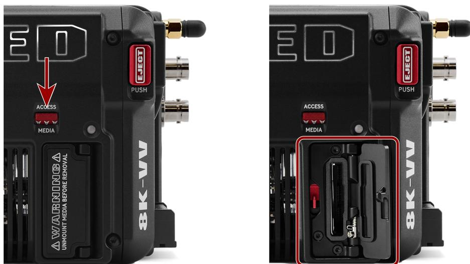
2. Insert the CFexpress media card in the slot with the top of the card facing toward the front of the camera. Insert the card until the lock clicks.
