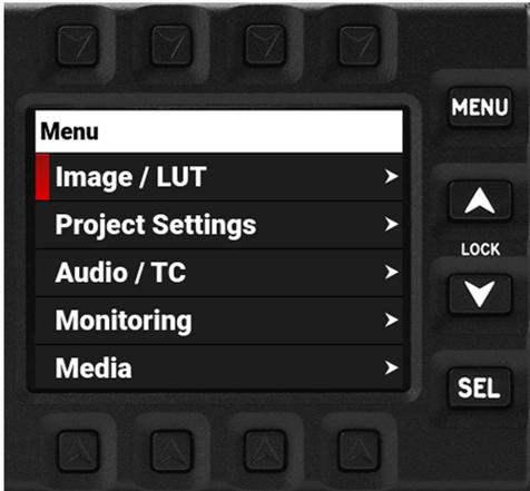
Press the up and down arrows to navigate up and down in the menu list. Press SEL to select a menu and open the submenus:
