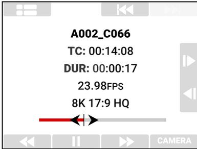
The Clip Information displays the name, Timecode, duration, project time base, format, and timeline of the clip.
