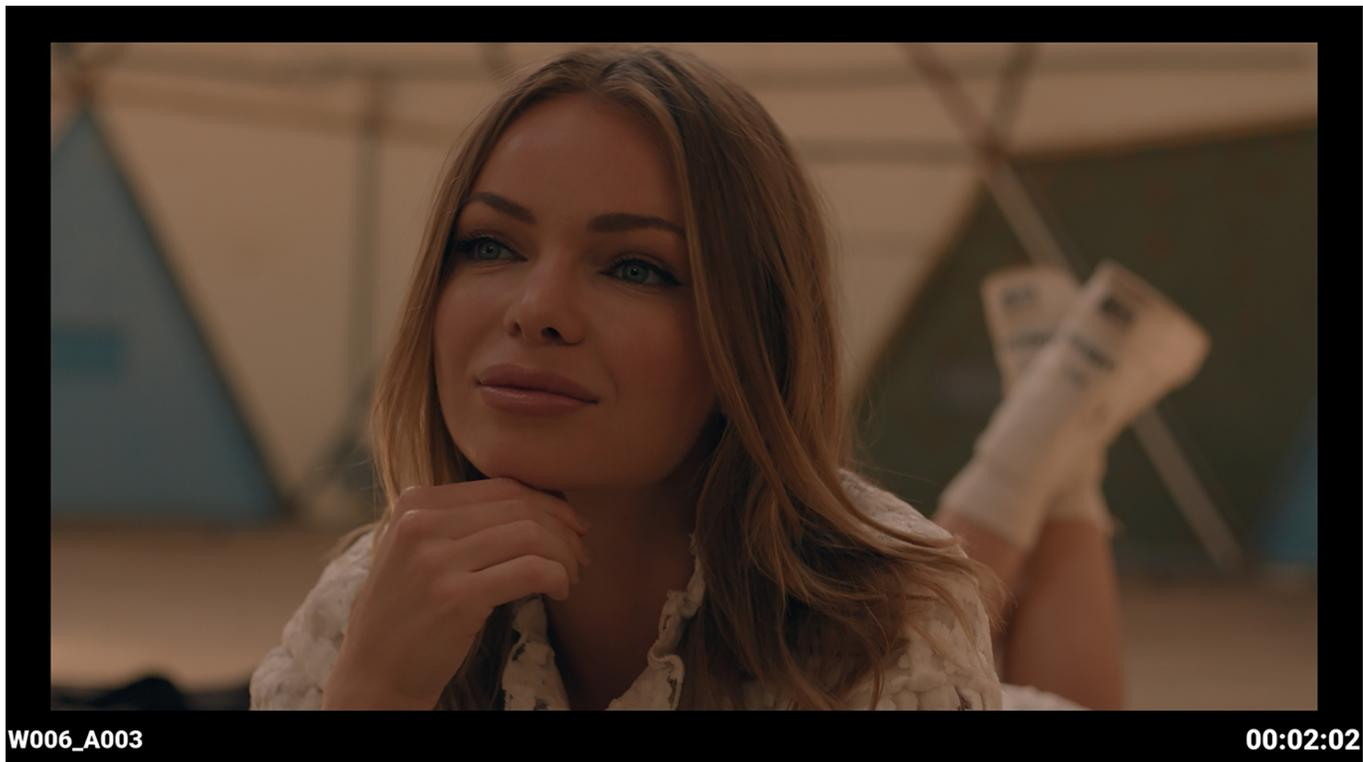
Simple mode displays the clip name and the current Timecode. When the camera is recording, the Timecode turns red, and a red dot appears in the top right corner.
