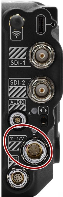
The male 6-Pin 1B DC-IN connector accepts DC input power from 11 V DC to 17 V DC. A built-in power conditioner protects against reverse-polarity connections, electrostatic discharge (ESD), undervoltage, overvoltage, and overcurrent.
