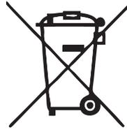
The Waste Electrical and Electronic Equipment (WEEE) mark applies only to countries within the European Union (EU) and Norway. This symbol on the product and accompanying documents means that used electrical and electronic products should not be mixed with general household waste. For proper treatment, recovery and recycling, take this product to designated collection points where it will be accepted free of charge. Alternatively, in some countries you may be able to return your
