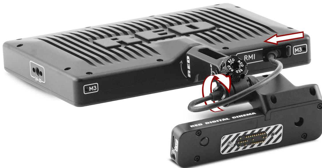
**NOTE:** The USB-C-style DSMC3 RMI cable is a custom-pinned cable, which is not compatible with standard USB-C cable ports.
