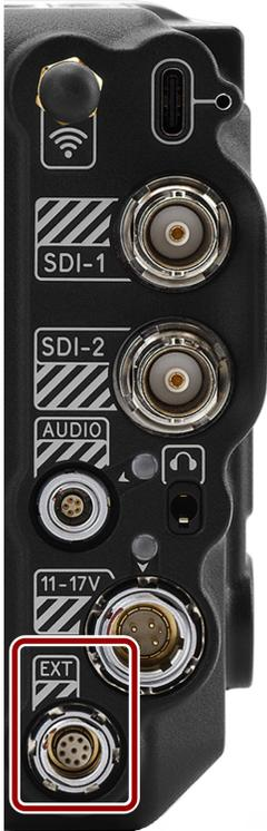
The female 9-contact 0B ODU Extension port supports serial (RS-232 RX and TX), a General Purpose Input (GPI) trigger (active-low switch closure), General Purpose Output (GPO), Timecode, and Genlock. The connector also offers auxiliary 5 Volt power out, with a maximum sustained current draw of 500 mA.
