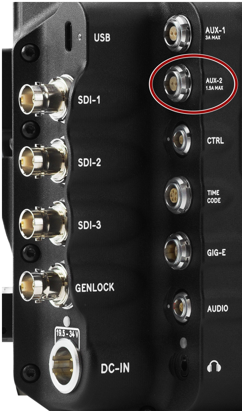
Figure: Front face of the AUX-2 female connector (looking at the back of the camera).
