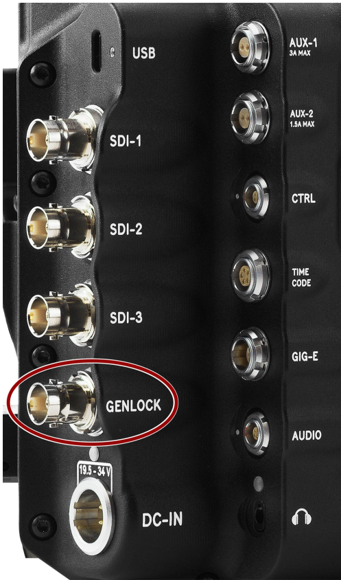
Figure: Front Face of the Genlock male BNC Connector (looking at the back of the camera).
