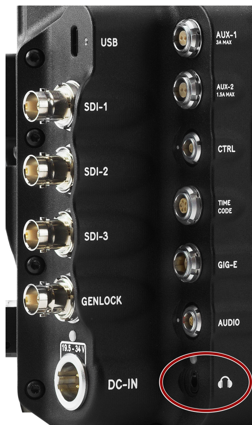
Figure: Front face of the female 3.5 mm headphone jack (looking at the back of the camera).
