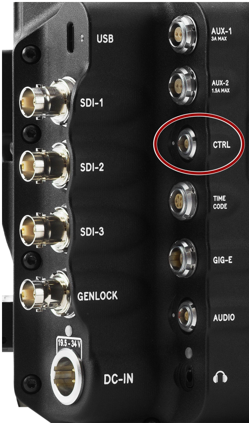
Figure: Front face of female 4-Pin 00B CTRL connector (looking at the back of the camera).
