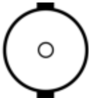
Figure: Front Face of the Genlock male BNC Connector (looking at the front of the connector).
