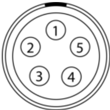
Figure: Front face of Timecode 0B Connector (looking at the front of the connector).
