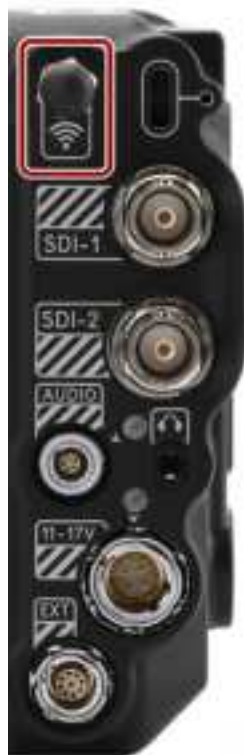
Figure: Front face of the female RP SMA port (looking at the back of the camera).
