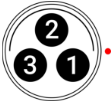
Figure: Front face of the female Fischer R/S connector (looking at the front of the connector).
