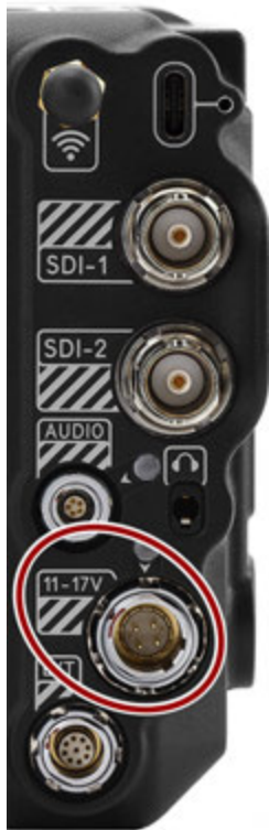
Figure: Front face of the male 6-Pin 1L DC power input connector (looking at the back of the camera).
