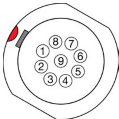
Figure: Front face of the female 9-contact Extension port (looking at the back of the camera).
