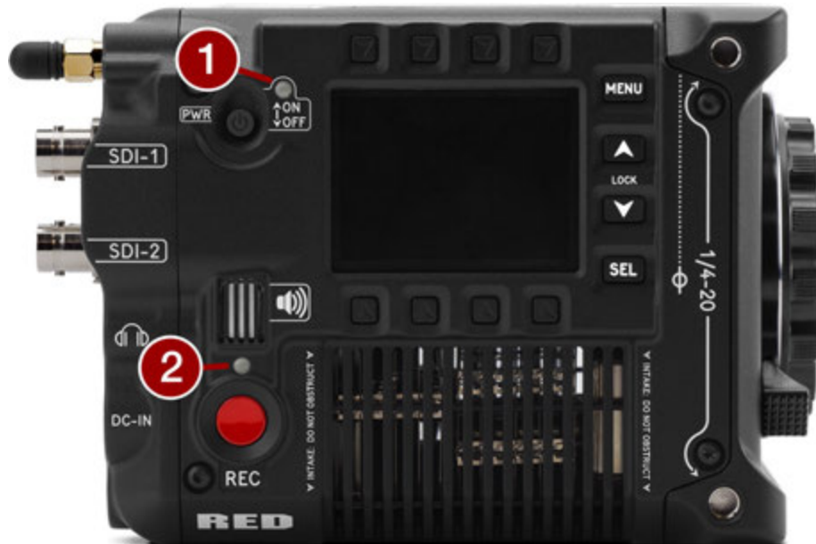
Figure: V-RAPTOR 8K VV LEDs, Right Side
