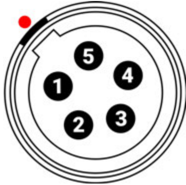
Figure: Front face of the female 5-Pin 00B audio connector (looking at the back of the camera).
