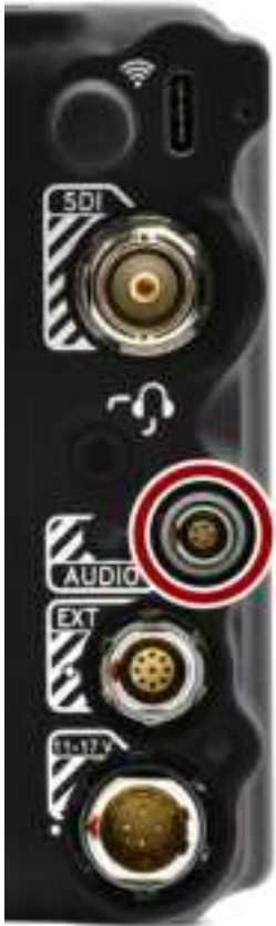
Figure: Front face of the female 5-Pin 00B audio connector (looking at the back of the camera).
