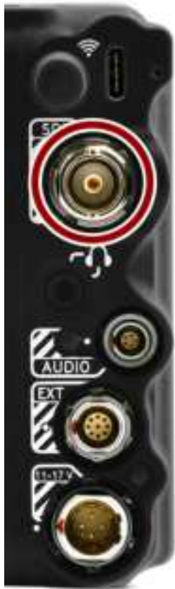
Figure: Front face of the 12G-SDI male BNC connector (looking at the back of the camera).
