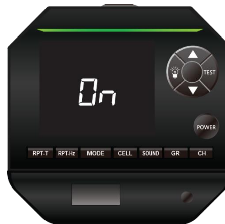
12. 'On' message appears on LCD display of flash.
