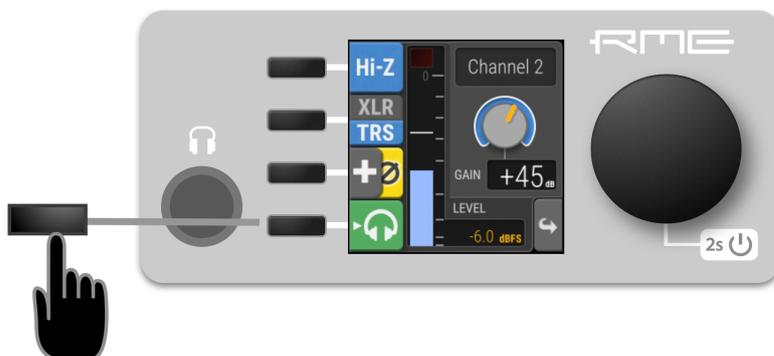
3. Use the fourth button to send this channel to the Phones Output (left and right) The button turns green, indicating that temporary routing has been established. The green button is also shown on the main screen and in the phones output settings.
