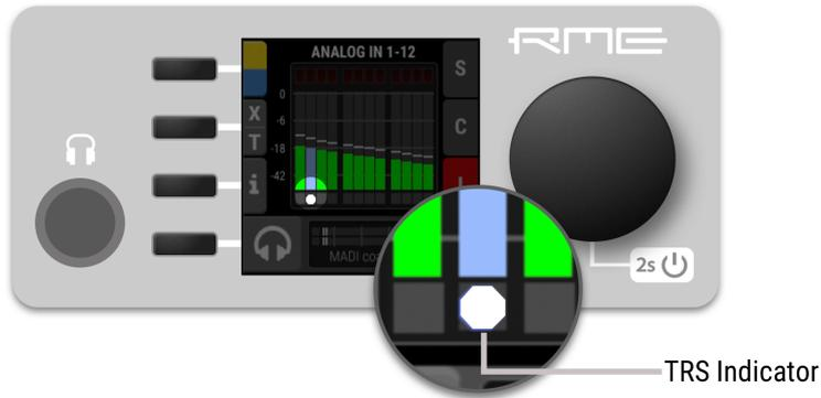
To toggle between XLR and TRS inputs on several channels:
