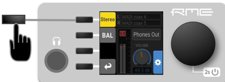
3. Press the "Stereo" button to separate the left and right channel. Each channel now has its own volume control which can be accessed by toggling the following button on the phones screen:
