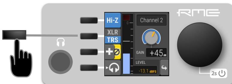
2. Use the **XLR|TRS** button to toggle the change the corresponding input. The active setting will be highlighted in blue.
