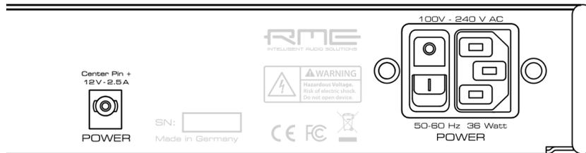
The **power switch** next to the inlet internally disconnects the line and neutral connection to the internal power supply. Ground will remain connected.
