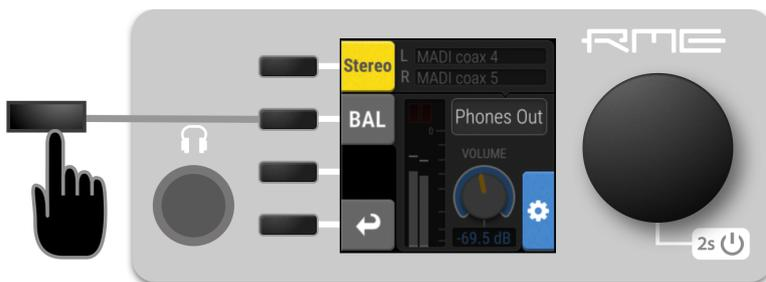
3. Press the "BAL" button to switch the channel to balanced out. The channel that was routed to the left phones output will now be applied to both tip and ring of a TRS connector, the phase being inverted on the ring.
