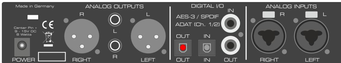
The rear panel of the ADI-2 FS features 2 servo-balanced analog inputs via XLR/jack combo jacks, 2 TS jacks as unbalanced outputs, 2 XLR jacks as balanced outputs, SPDIF I/O via TOSLINK optical and RCA coaxial, and a lockable power supply jack.
