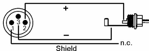
The ground-free design with transformer in the coaxial input offers full compatibility to AES/EBU along with perfect hum rejection.
