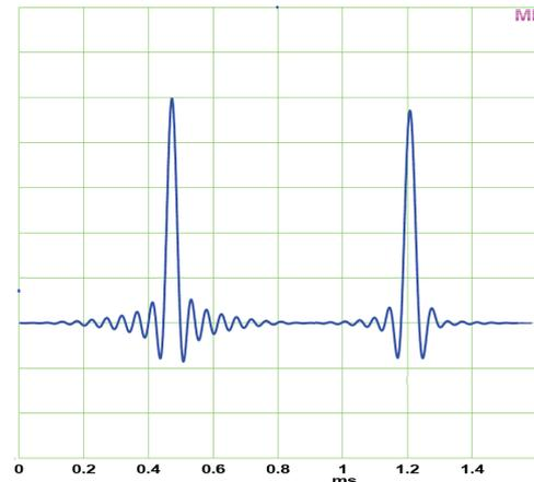
SD Slow and Slow work best at 88.2/96 kHz, because the decrease in the high frequency area then happens outside the audible range. At the same time the impulse response is near perfect – caused by both the filter as well as the doubled sample rate.
