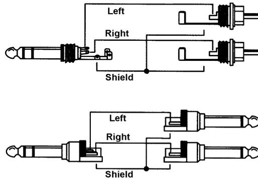
RME has a history of phones outputs working perfectly as line outputs. The Extreme Power phones outputs of the ADI-2 Pro continue this legacy by delivering exceptional performance with widest compatibility and versatility. For example turning on Balanced Phones mode, the two TRS jacks on the front perfectly serve as high-quality TRS balanced line outputs.
