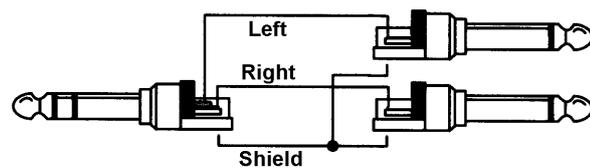
In Balanced Mode operation the TRS outputs change from unbalanced stereo to balanced mono operation. An adapter cable as shown to the right gives balanced phones with 4-pin XLR connector access to the ADI-2 Pro outputs.
