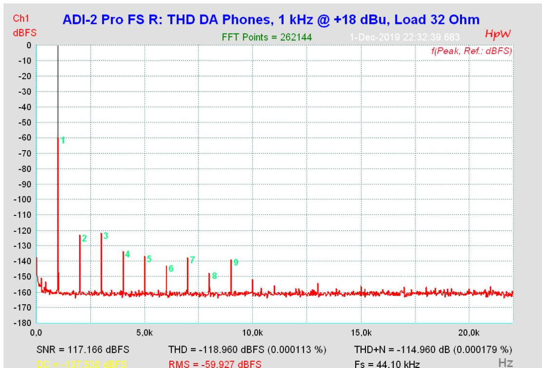
\*\* Measured with active notch filter via ADC of ADI-2 Pro FS. +18 dBu output level @ 32 Ohm equal 1.2 W (per channel)
