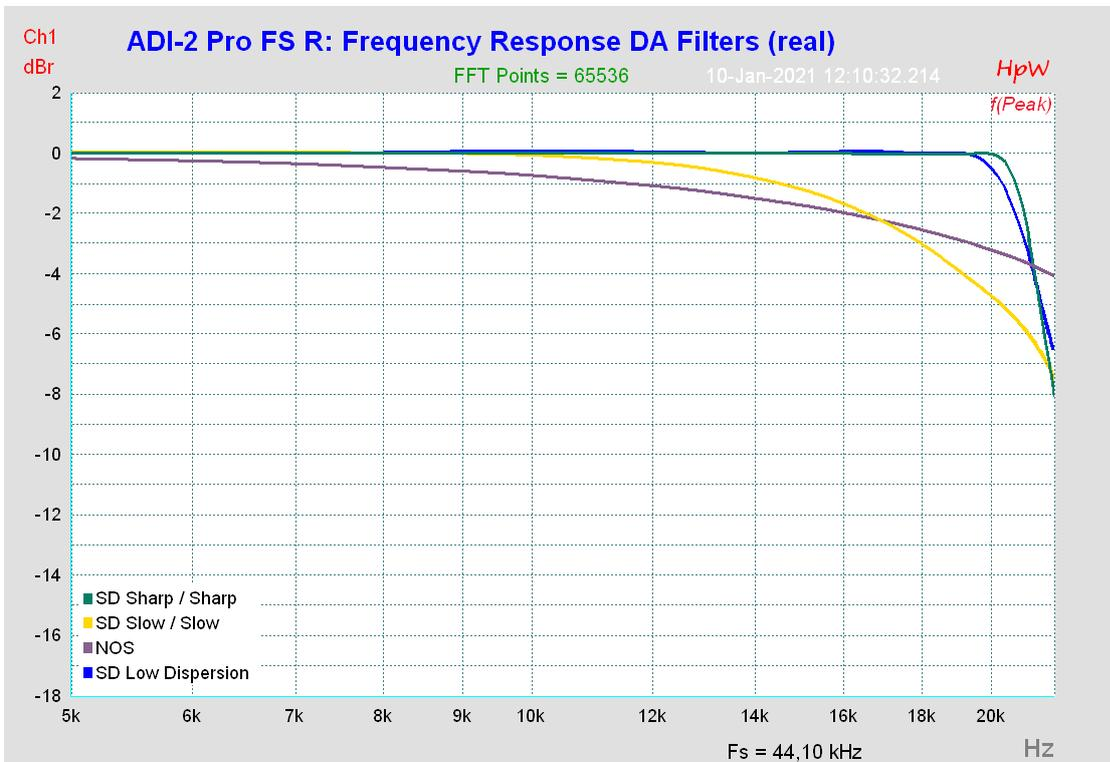
**Note:** Sharp/SD Sharp and Slow/SD Slow are congruent. NOS shows a very early drop. SD Low Dispersion is almost as linear as Sharp/SD Sharp.
