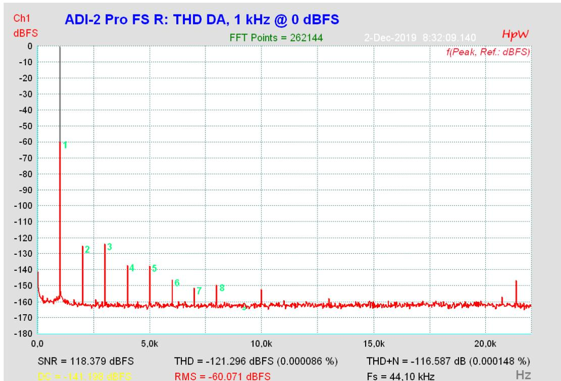
\* Measured with active notch filter via ADCs of ADI-2 Pro FS in mono mode (M/S)
