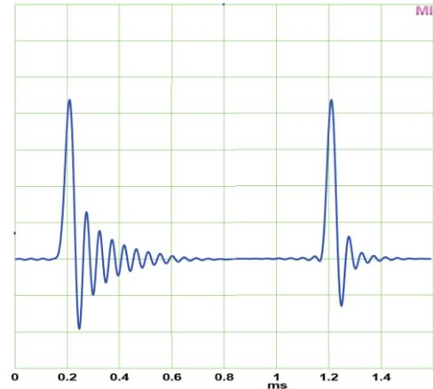
In the picture to the right the impulse responses of filters *Sharp* (left) and *Slow* (right) are shown, again at 44.1 kHz. Sharp generates the expected, Slow a near perfect impulse response.
