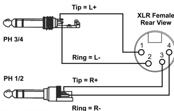
The use of a 4-pin XLR male connector on the phones side is quite popular. The diagram to the right shows how an adapter cable can be used to connect the ADI-2 Pro phones outputs, using two stereo TRS plugs and one female XLR connector.
