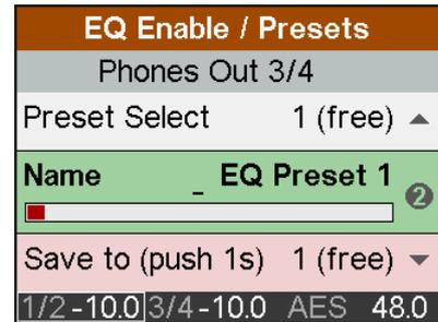
Leaving this field the name is automatically adjusted to the right. Adding signs to the front and rear is possible afterwards. A quick turn to the left brings up space, which is also used to quickly delete letters. Available signs are:
