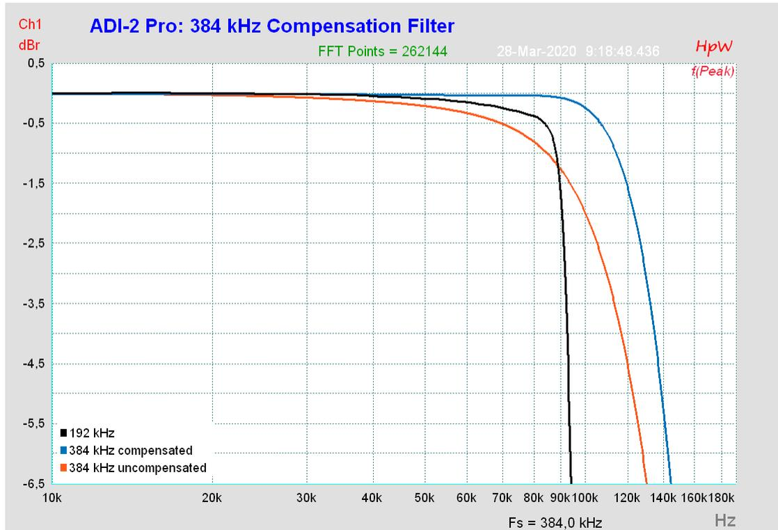
The blue curve shows the effect of RME's digital compensation filter at 384 kHz sample rate. The frequency response is now near flat up to 90 kHz, with minimal decrease in the area of the 192 kHz sample. With this filter the ADI-2 Pro can easily measure any 192 kHz (and lower, of course) operated device with high accuracy, at fractions of a dB.
