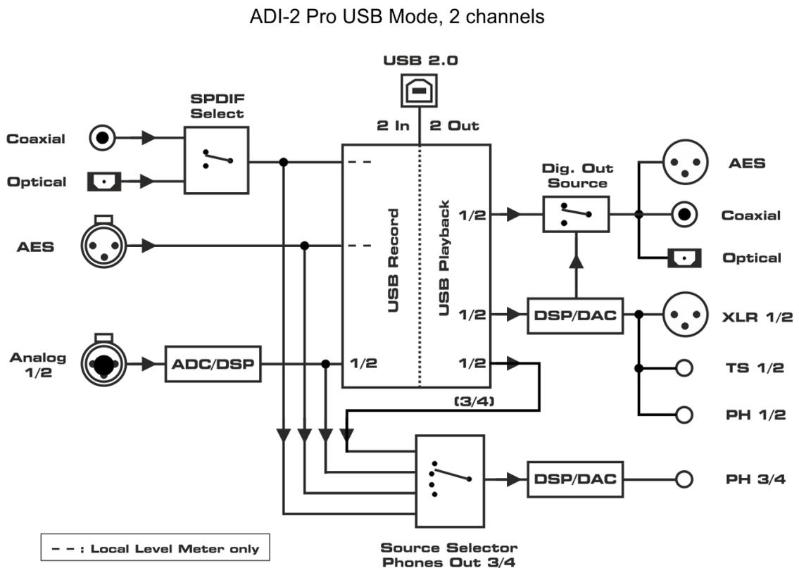
USB Playback channels 3/4 can only be monitored in multi-channel mode. In stereo mode selecting USB 3/4 plays channels 1/2.
