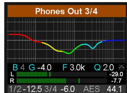
Another push on encoder 2 changes to the graphical EQ Preset selection screen. Turning encoder 2 will scroll through all available EQ presets with the frequency graphics showing the respective curve, and the parameter line showing the preset name. In this screen Volume, volume selection and channel selection (encoder 1) are also available.
