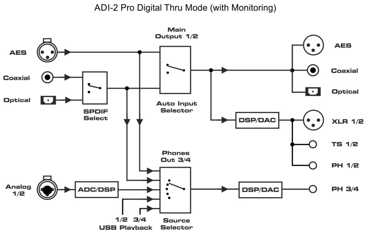
Note: To simplify the diagram and to maintain overview USB record is not shown. In all modes all input signals are sent over USB to the host. In multi-channel mode three separate stereo pairs, in stereo mode only the stereo analog input.
