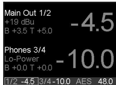
Despite this screen having no level meters, overloads caused by Volume, PEQ or Bass/Treble are easy to recognize. The big gain numbers are coupled to the over detection of the analog outputs. They change their color to red when overload occurs.
