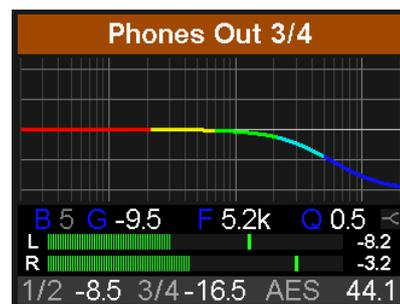
For an inverted filter curve select band 5 with type shelf active, set Q to 0.5, Frequency to 5.2 kHz and Gain to -9.5 dB. Similarly, a pre-emphasis is done with the same settings but Gain to +9.5 dB.
