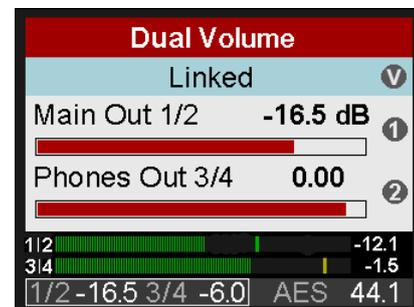
In the Dual Volume screen, both outputs can be muted by pushing encoder 1 (B) and encoder 2 (T) respectively.
