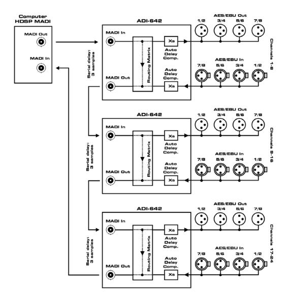
Playing back a test signal on all 64 channels of the MADI card simultaneously, the signals will be delayed at the outputs of the second ADI-642 by 3 samples, at the third by 6 samples and so on. At Double Speed the delay rises to 6 samples per unit, at Quad Speed to 12 samples.
