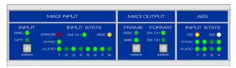
The MADI output signal can include 56 or 64 channels (FORMAT). The FRAME key switches the MADI output into native Double Speed mode (96K), in case internal or external clock allow this mode to be activated.
