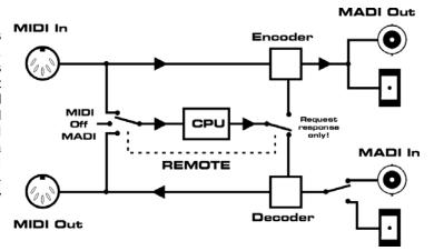
The MIDI input signal will never be transferred directly from MADI to MADI, no matter how the matrix router is set up. A MIDI cable connecting MIDI output and MIDI input of the ADI-6432, will realize a direct pass-through of MIDI, from MADI input to MADI output.
