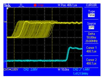
The cleaned and jitter-freed signal can be used as reference clock for any application, without any problem. The signal processed by SteadyClock is of course not only used internally, but also available at the ADI-6432's word clock output. It is also used to clock the digital outputs MADI and AES/EBU.
