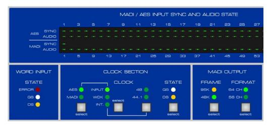
In the CLOCK SECTION the current clock reference and frequency multiplier is chosen.
