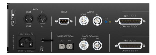
**IEC receptacle** for power connection. The specially developed, internal hi-performance switch mode power supply makes the ADI-6432 operate in the range of 100V to 240V AC. It is short-circuit-proof, has an integrated line filter, is fully regulated against voltage fluctuations, and suppresses mains interference.
