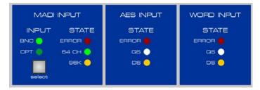
**AES INPUT** displays the basic state of the AES input signal: ERROR, Double Speed and Quad Speed. The big LED display, **AES INPUT STATE**, shows the presence of a valid input signal separately for each AES input. RME's exclusive *SyncCheck* indicates via flashing LEDs if one of these inputs is locked, but not synchronous to the chosen clock reference.
