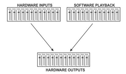
TotalMix can be used in the above view (View Options **2 Rows**). However, the default is a vertical alignment in three rows as known from an Inline desk, so that the row *Software Playback* equals the *Tape Return* of a real mixing desk:
