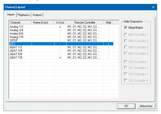
Hidden channels in *MIDI Remote x* are removed from the list of remote controllable channels. Within an 8-channel block of a Mackie compatible control they are skipped. The control therefore is no longer bound to consecutive orders. For example it will control channels 1, 2, and 6 to 11, when channels 3 to 5 are hidden. The same can be done for OSC. With unnecessary channels made invisible for the OSC remote the more important channels are available as one block on the remote.
