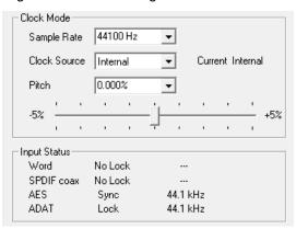
This way, configuring any suitable audio application for digital recording is simple. After selecting the correct input, Fireface UCX II displays the current sample frequency. This parameter can then be changed in the application's audio attributes (or similar) dialog.
