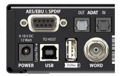
**DURec (Remote).** Connector for USB stick or USB hard drive. Offers direct recording to / play-back from the external memory device. Alternatively connector for the optional Advanced Remote Control USB (ARC USB) when the UCX II is used in stand-alone and Class Compliant mode. This port can also be used instead of connecting the ARC USB to the computer.
