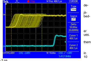
The screenshot shows an extremely jittery SPDIF signal of about 50 ns jitter (top graph, yellow). SteadyClock turns this signal into a clock with less than 2 ns jitter (lower graph, blue). The signal processed by SteadyClock is of course not only used internally, but also used to clock the digital outputs. Therefore the refreshed and jitter-cleaned signal can be used as reference clock without hesitation.
