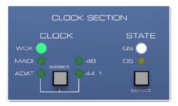
A selection of DS and QS is also possible when using external clock (Slave). If the M-32 DA should operate at 192 kHz, but receives a synchronous word clock of 48 kHz, the button STATE activates DS or QS mode. This way, AD-conversion and digital outputs are configured to operate in the frequency ranges Single Speed, Double Speed or Quad Speed.
