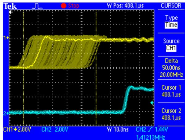
The cleaned and jitter-free signal can be used as reference clock for any application, without any problem. The signal processed by SteadyClock is of course not only used internally, but also available at the Micstasy's word clock output. It is also used to clock the digital outputs MADI and AES/EBU.
