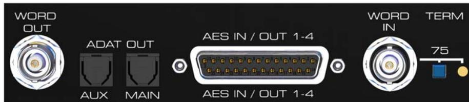
**WORD IN (BNC):** A push switch allows to activate internal termination (75 Ohms).
