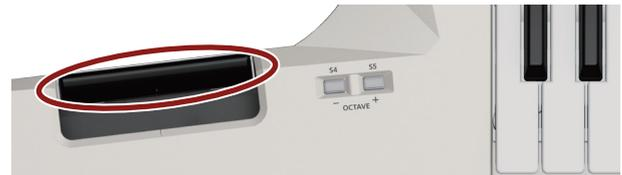
\* The effect applied by the **MODULATION BAR** differs depending on the setting. Normally, pressing the **MODULATION BAR** applies a vibrato effect. To change the setting, refer to **"Assigning the Function of Each Controller"** (p. 12).
