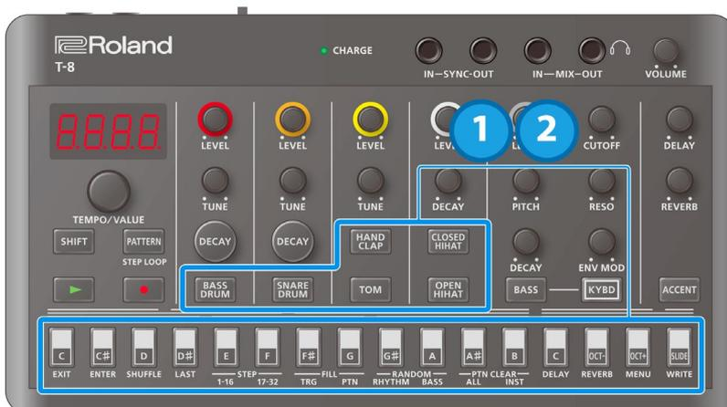
1. Hold down an instrument button and press one of the step 1–16 buttons.
