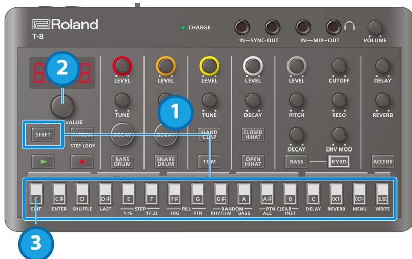
1. Hold down the [SHIFT] button and press the step button corresponding to the function you want to execute.
