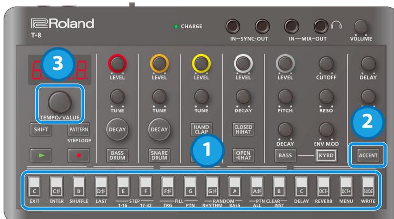
1. **Press one of the step 1–16 buttons (and keep holding the step buttons until the operation is finished).**
