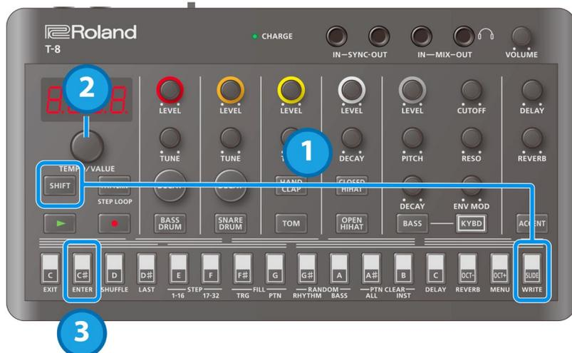
1. Hold down the [SHIFT] button and press the [SLIDE (WRITE)] button.
