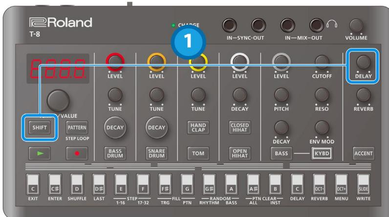
1. Hold down the [SHIFT] button and turn the [DELAY] knob.
