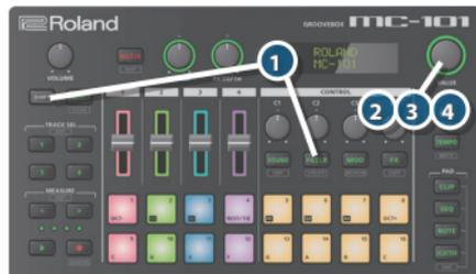
1. Hold down the **[SHIFT]** button and press the **[FILTER]** button.
