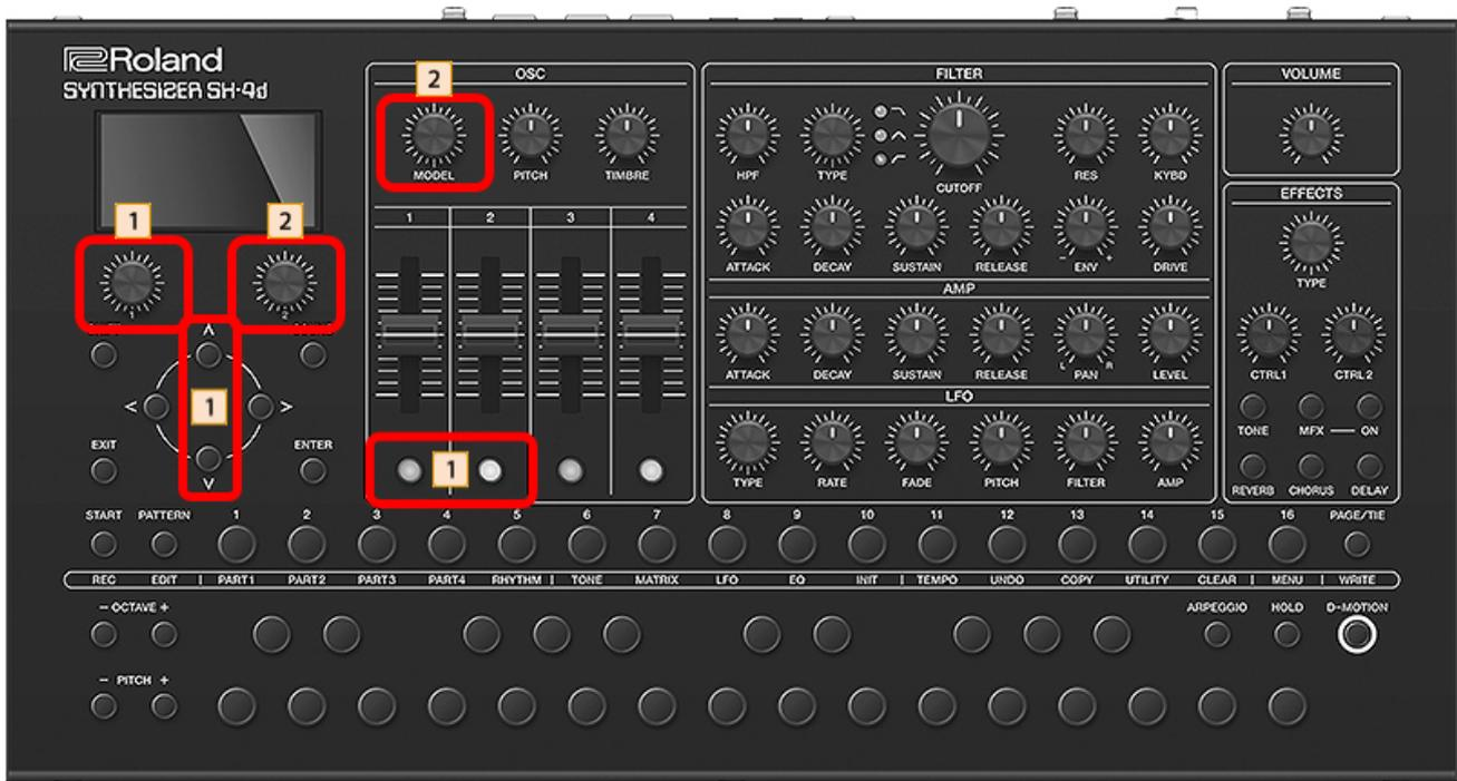
1. Use the [1] knob, [^] [v] or [OSC 1] [OSC 2] buttons to select the layer for which you want to choose a waveform.
