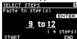
Use the [1] knob or the [2] knob to select the starting step number, and press the [ENTER] button to execute the paste operation.
