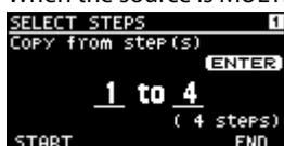
Use the [1] knob to select the starting step and the [2] knob to select the ending step number, and press the [ENTER] button to execute the copy operation.
