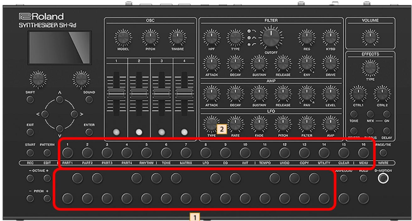
1. Press a keyboard button to select the instrument you want to input.
