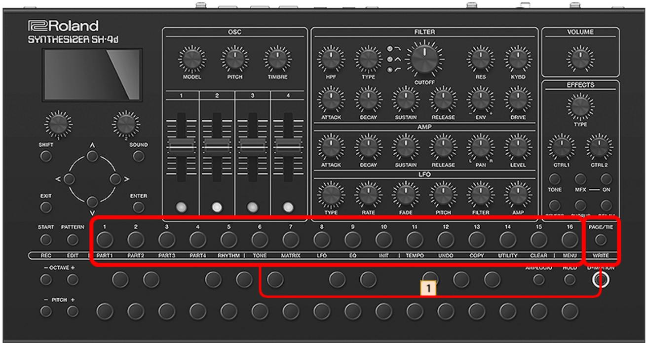
1. Hold down one of the [1]–[16] buttons corresponding to where you want the tie to start, and press the [PAGE/TIE] button.
