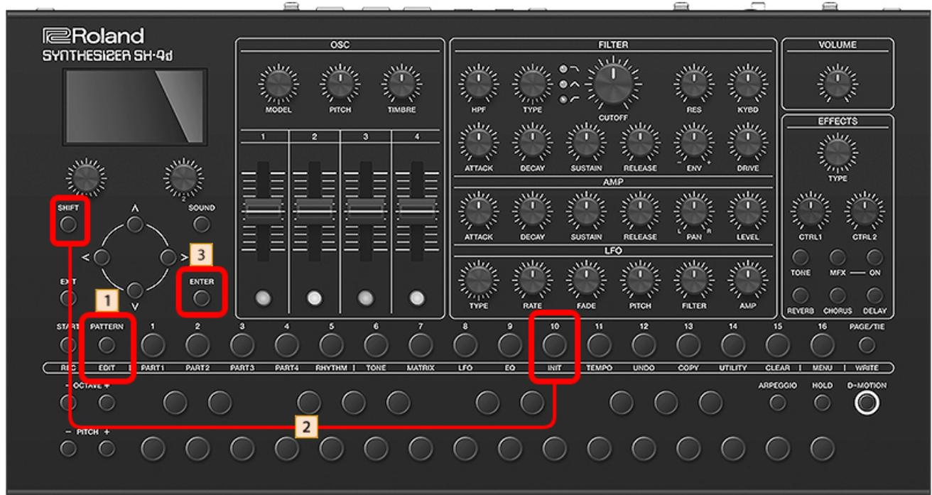
1. Press the [PATTERN] button to display the PATTERN screen, and select the pattern to initialize.
