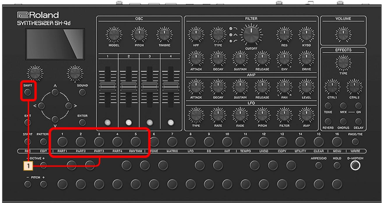
1. Hold down the [SHIFT] button and press the [1]–[5] buttons.
