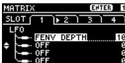
If no slots are available, the message "No empty slot" appears, and the display automatically switches to the MATRIX screen. Try changing the settings on the MATRIX screen to a different slot or destination that has already been set.
