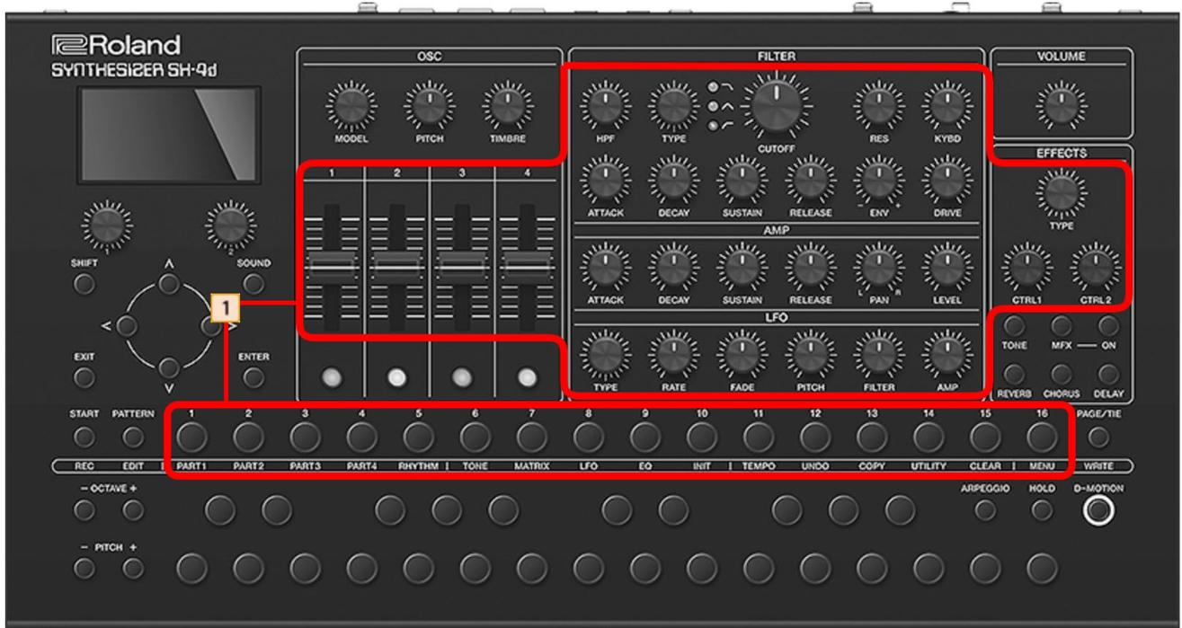
1. Hold down the respective [1]–[16] buttons while turning the knob of the selected step where you want to save the motion, and set the value.
