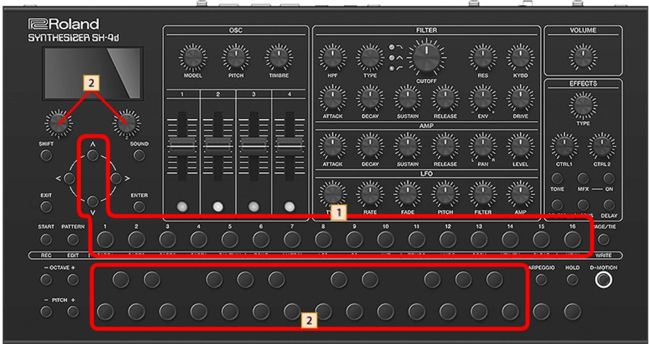
1. Long-press the [1]–[16] buttons to bring up the STEP EDIT screen. While holding down the [1]–[16] buttons, press one of the [^] [v] buttons.
