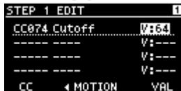
When you play back the step sequencer, the values for the knobs change according to the values recorded for each step.
