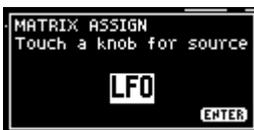
3. Operate the controller (knob, slider or button) corresponding to the source/destination you want to set.
