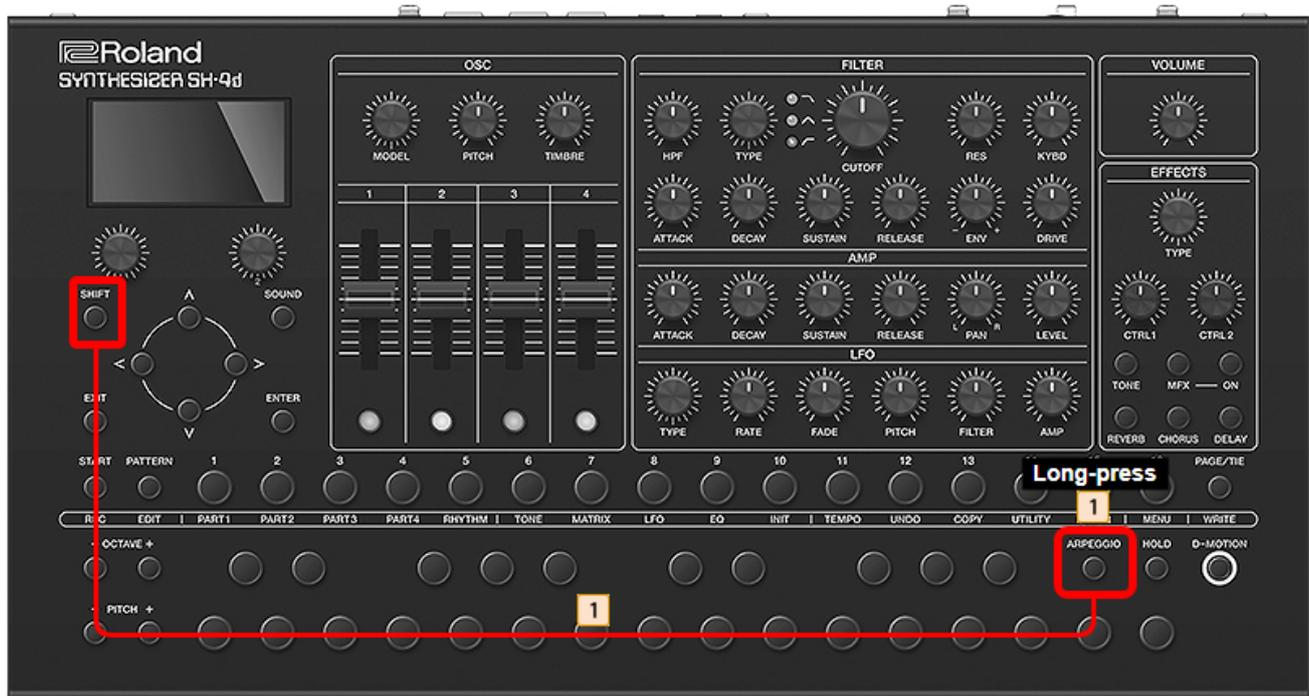
1. Long-press the [ARPEGGIO] button, or hold down the [SHIFT] button and press the [ARPEGGIO] button.
