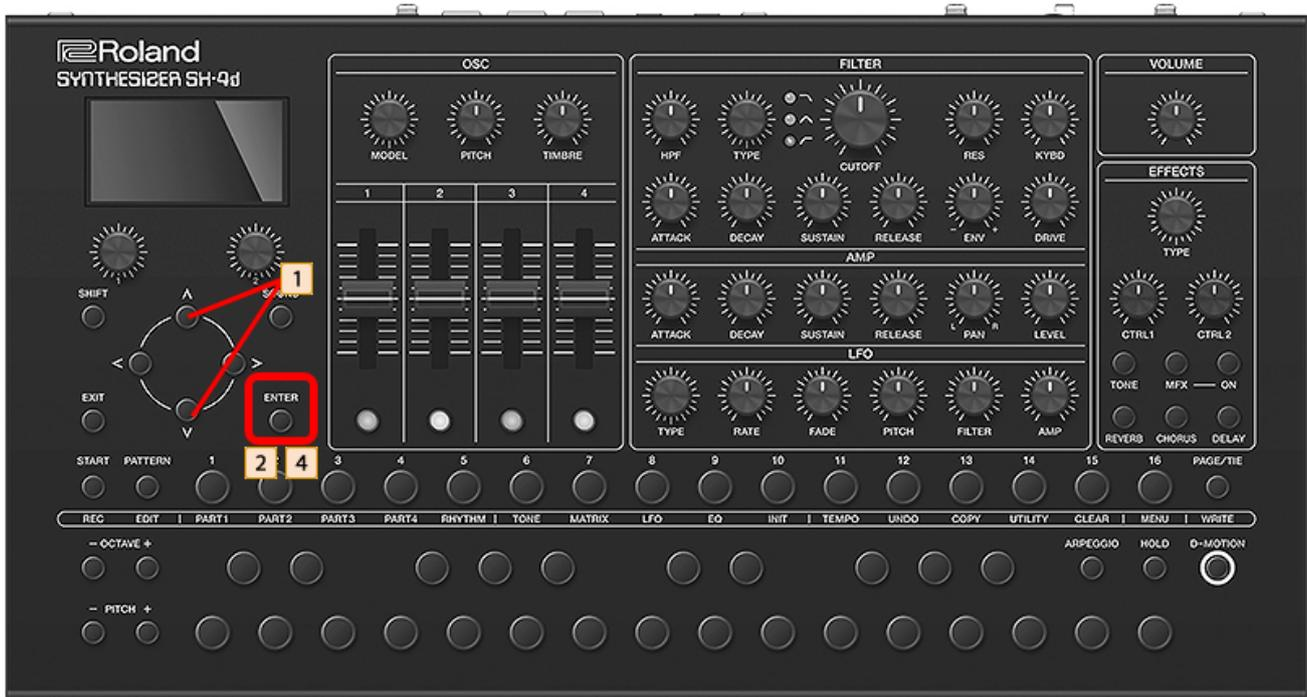
1. On the MATRIX screen, press the [▲] [▼] buttons to select the source/destination to edit.
