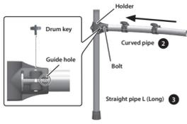
2-3. Use the drum key to loosen the bolt of the drum sound module holder, then attach the drum sound module holder to straight pipe "L" (long) 3 and tighten the bolt.
