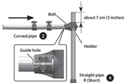
2-6. Position straight pipe "R" (short) 4 so that its tip protrudes by about 7 cm (3 inches), and then tighten the holder.
