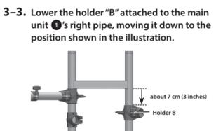
3-3. Lower the holder "B" attached to the main unit 1's right pipe, moving it down to the position shown in the illustration.
