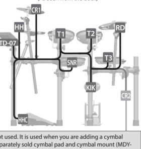
\* "CR2" is not used. It is used when you are adding a cymbal using a separately sold cymbal pad and cymbal mount (MDY-Standard). If you are not adding this, leave the cap attached. Fasten it so that it does not obstruct your performance.
