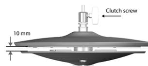
\* Although the gap can be adjusted to a clearance that makes playing the hi-hat easier, setting too narrow or wide a gap can cause improper function of the unit and prevent the hi-hat from sounding as you intend. Setting the gap to 10 mm provides the most natural feel when playing the VH-14D.
