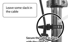
2. Wind a cable tie around the pipe and tighten it in order not to slip.
