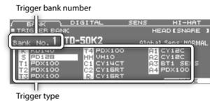
4. Place the cursor on the trigger bank number, and use the [-] (+) buttons or the dial to set the trigger bank to "TD-50KV2."
