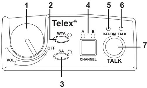
1. **On/Off & Volume Control** - Turns the belt-pack power on and controls headset volume.
