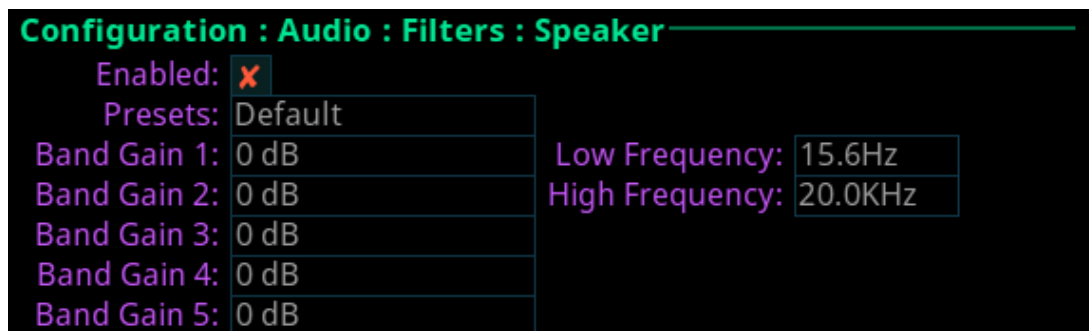
Figure 23.7: Configuration | Audio | Filters | Speaker
