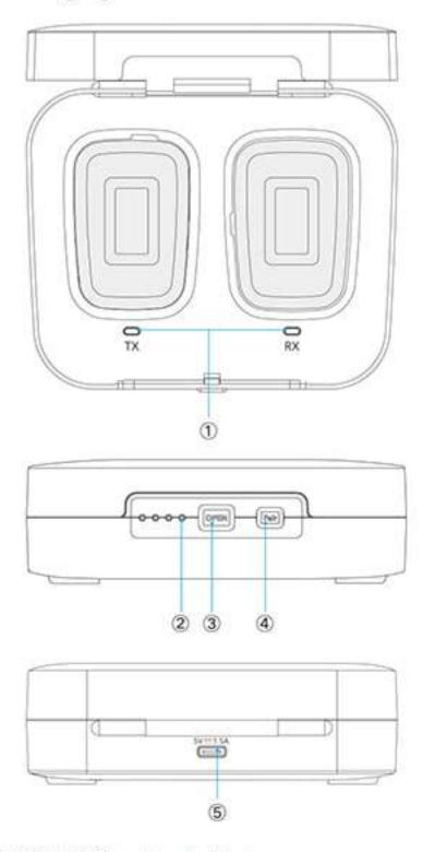
① TX & RX Charging Indicator Charging =Solid Red Fully Charged=Lights Off
