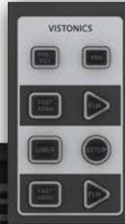
The Master Bay VISTONICS button group [PAGE A] and [PAGE B] buttons determine which bus master range is controlled by the encoders Master Bay VST encoders.
