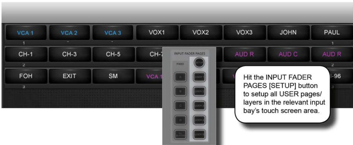
Hit the INPUT FADER PAGES [SETUP] button to setup all USER pages/ layers in the relevant input bay's touch screen area.
