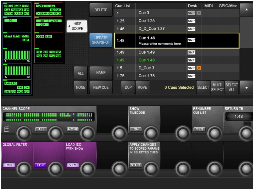
It can be very useful to make a Cue which, when it is recalled, only affects a specific area of the console - a 'Partial' snapshot. For example, you could make cues that will only set the Gains and EQ of all the channels, but leave the fader values unchanged.
