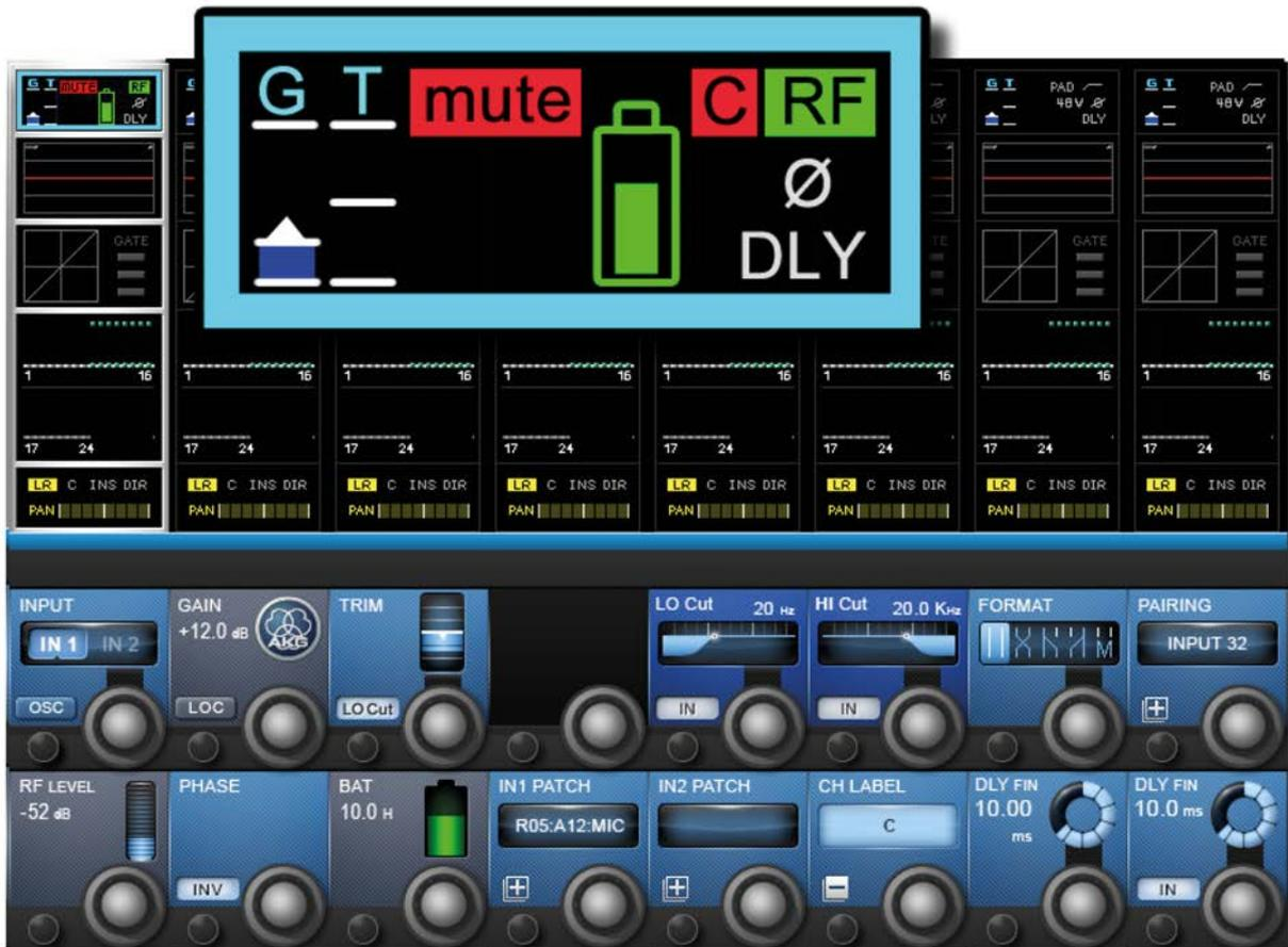
The console displays VM<sup>2</sup> wireless system status information in two places - the main channel strip display in the input channel touch screen area (input block), and in the VST area when the channel's input block has been selected.
