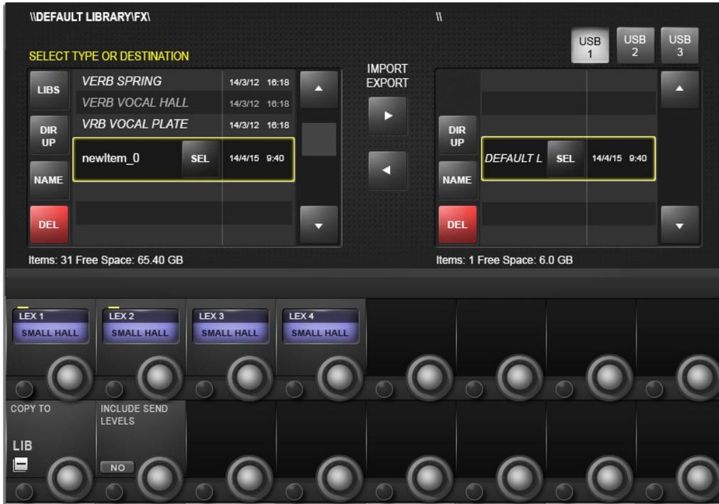
The Library file system appears in the Master Bay Visonics screen when the {LIB} button is pressed in Copy or Paste Mode. It allows you to navigate the console library and perform import/export operations with connect USB storage devices.
