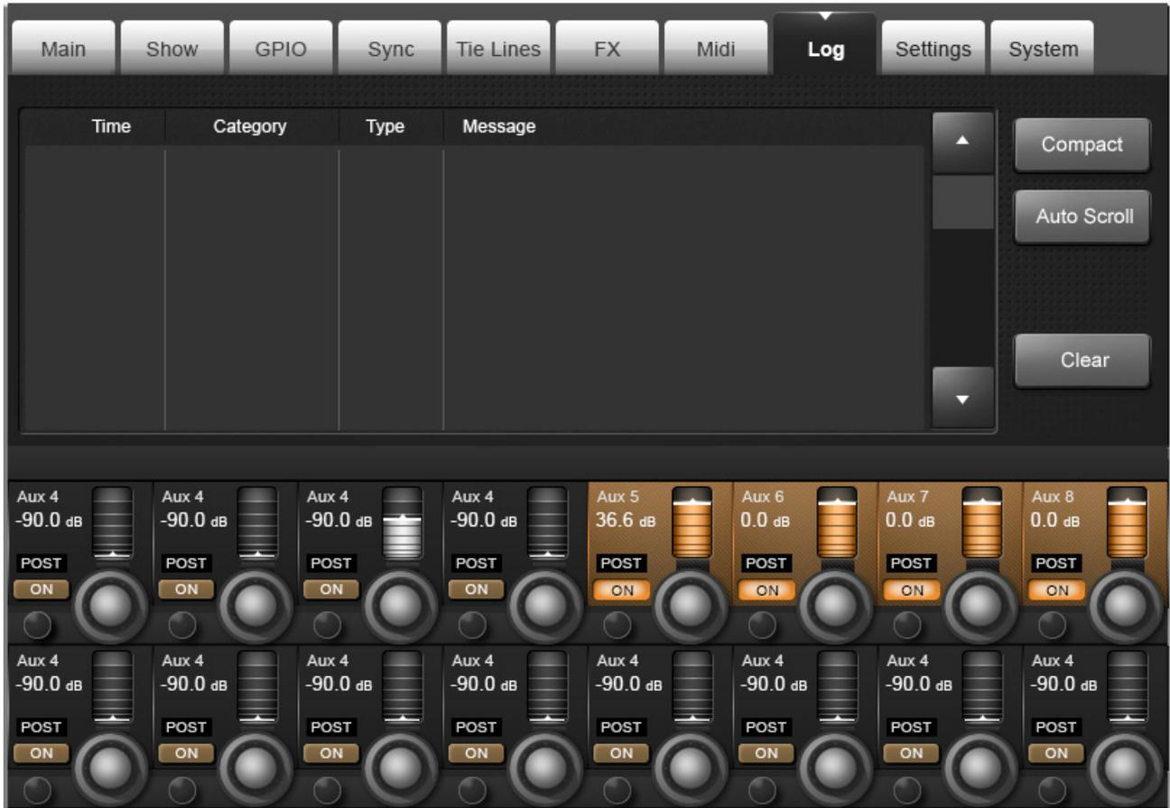
This page displays any errors that have occurred since the console was last powered-up. These would usually be communications errors between the various components in the system such as control surface, local rack, and stagebox.
