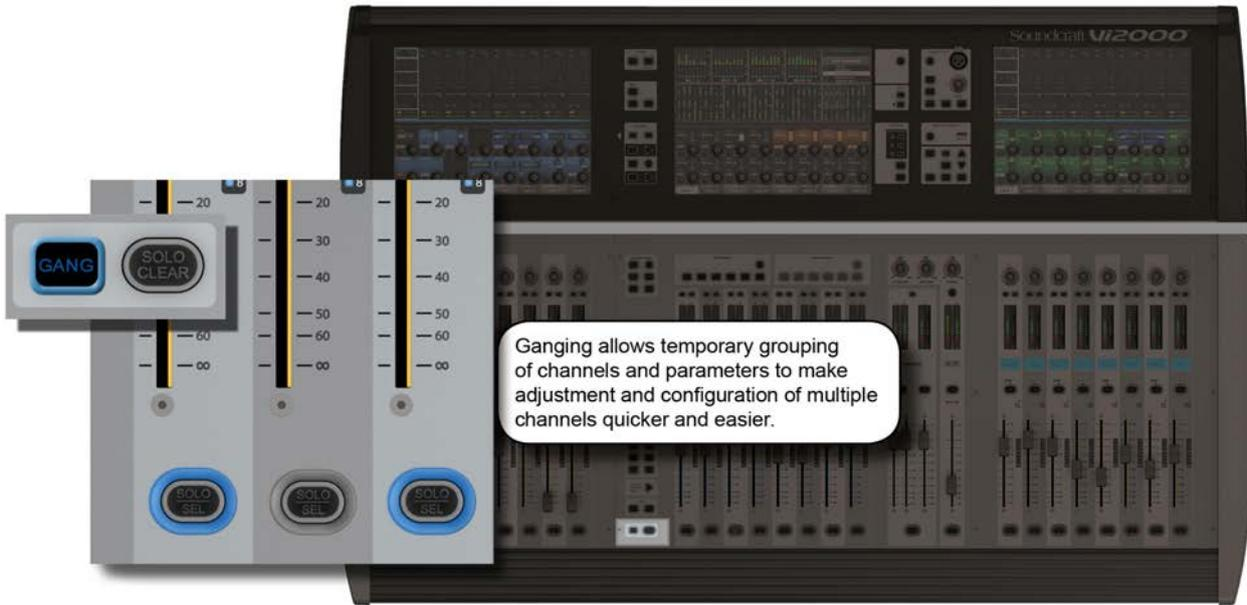
Gang is a very helpful feature to speed up operations that influence functions on multiple input channels, or on output busses, in the same way. Any parameter change on ganged channels will be applied to all other ganged channels as an offset. For example, adding 4dB of level to an aux send on one channel will add 4dB of level to the the corresponding Aux sends on all other ganged channels - it will not 'copy' the actual level to the other ganged channels.
