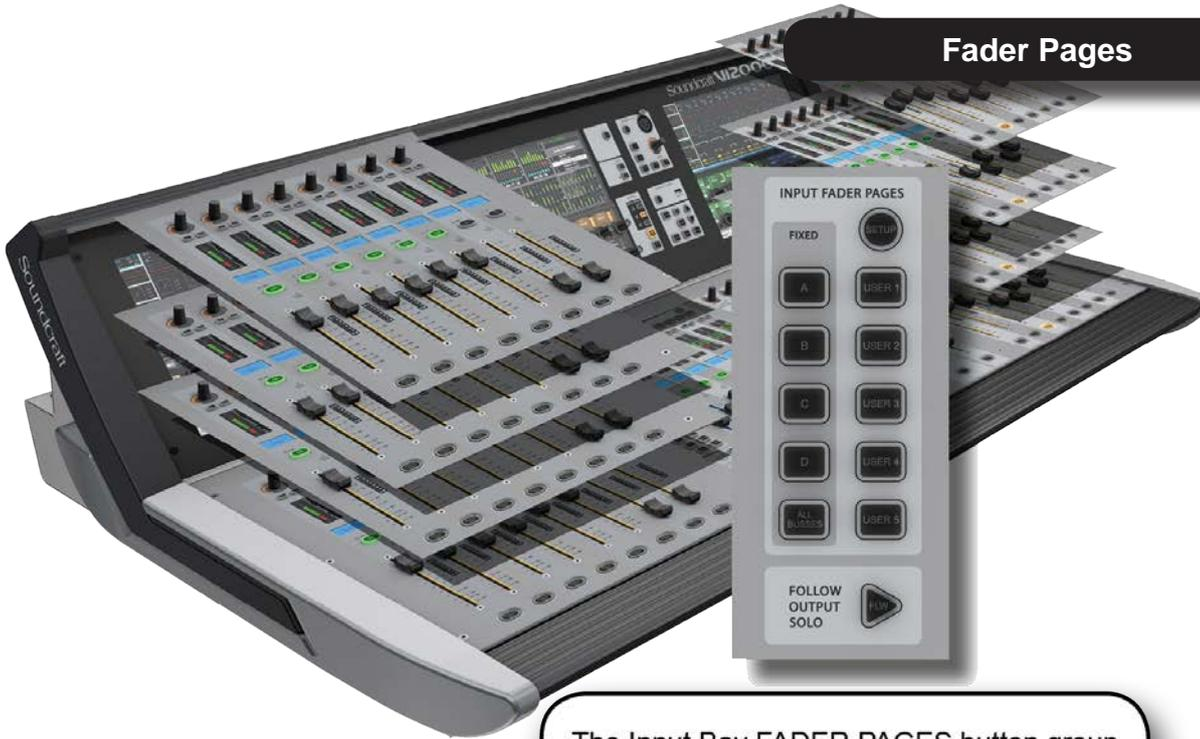
The Input Bay FADER PAGES button group enables rapid selection and setup of preset and user-configured Fader pages (layers).
