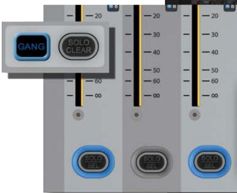
Ganging allows temporary grouping of channels and parameters to make adjustment and configuration of multiple channels quicker and easier. To Gang channels, hit the [GANG] button then add or subtract channels with their [SOLO/SEL] buttons.
