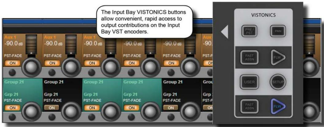
These buttons control the functionality of the input channel VST encoders.
