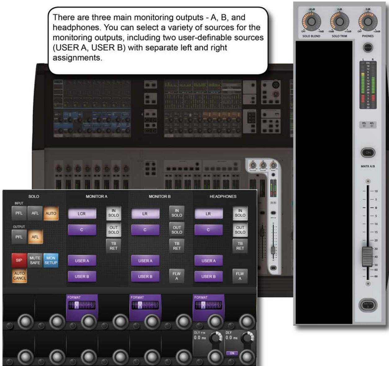
The monitoring system has three main sources - Monitor A, Monitor B, and Headphones. These are fed by a choice of sub-sources, including Solos, LCR, Talkback return, and two user-defined stereo sources where the left and right signals can be patched independently
