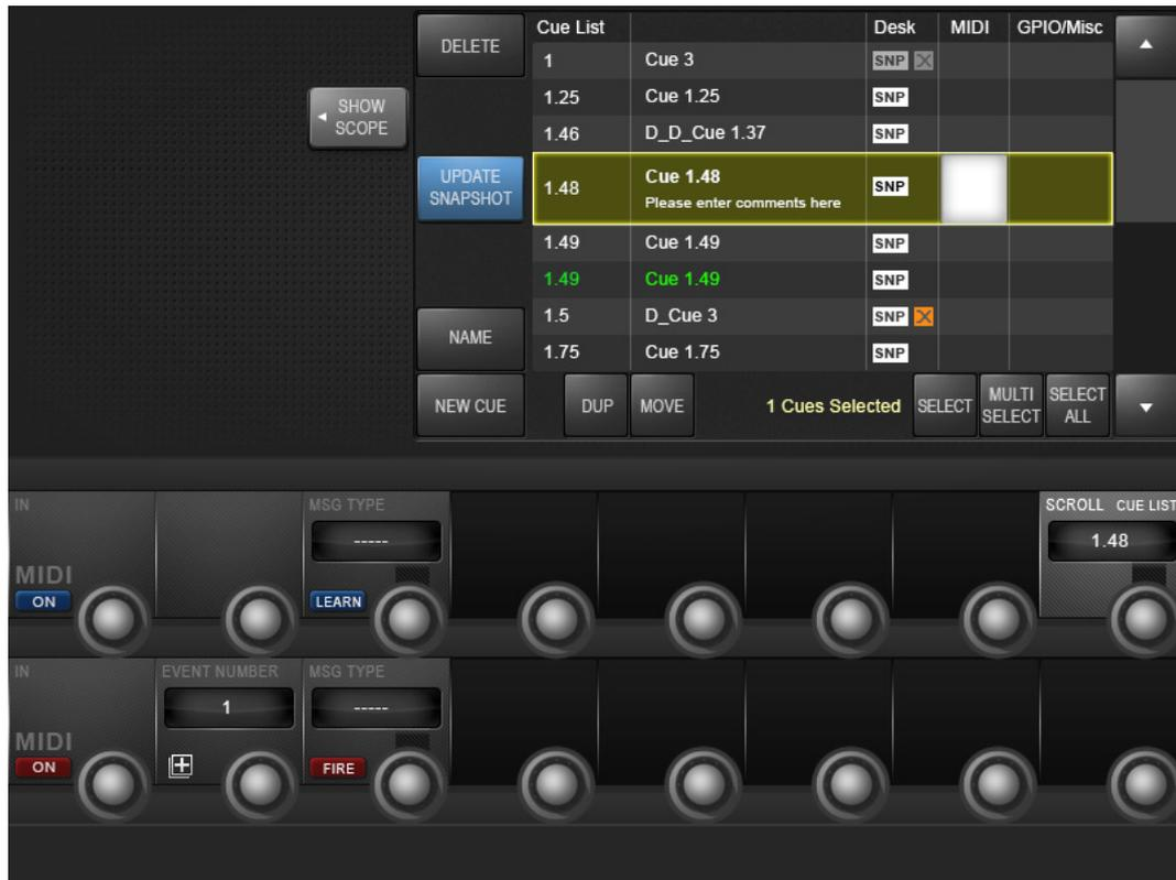
Selecting the MIDI column in a cue list entry gives access to that cue’s MIDI input trigger and output settings. The output section defines an event list of MIDI messages that are sent when the cue is triggered. Note that some options rely on, or are governed by, global MIDI settings, accessed via the Settings menu.
