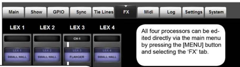
All four processors can be edited directly via the main menu by pressing the [MENU] button and selecting the 'FX' tab.
