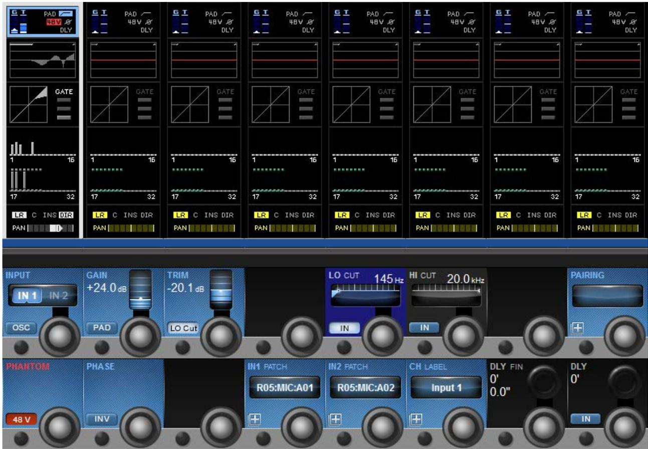
A mono input channel's input section touch screen area is at the top of the Vistonics input channel strip area, colour-coded blue. The input section consists of that channel's input source selection, pre-amp and gain stages control, channel pairing selection for stereo (and other format) channel creation, channel labelling, and channel delay adjustment.
