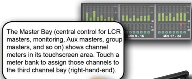
The Master Bay (central control for LCR masters, monitoring, Aux masters, group masters, and so on) shows channel meters in its touchscreen area. Touch a meter bank to assign those channels to the third channel bay (right-hand-end).
