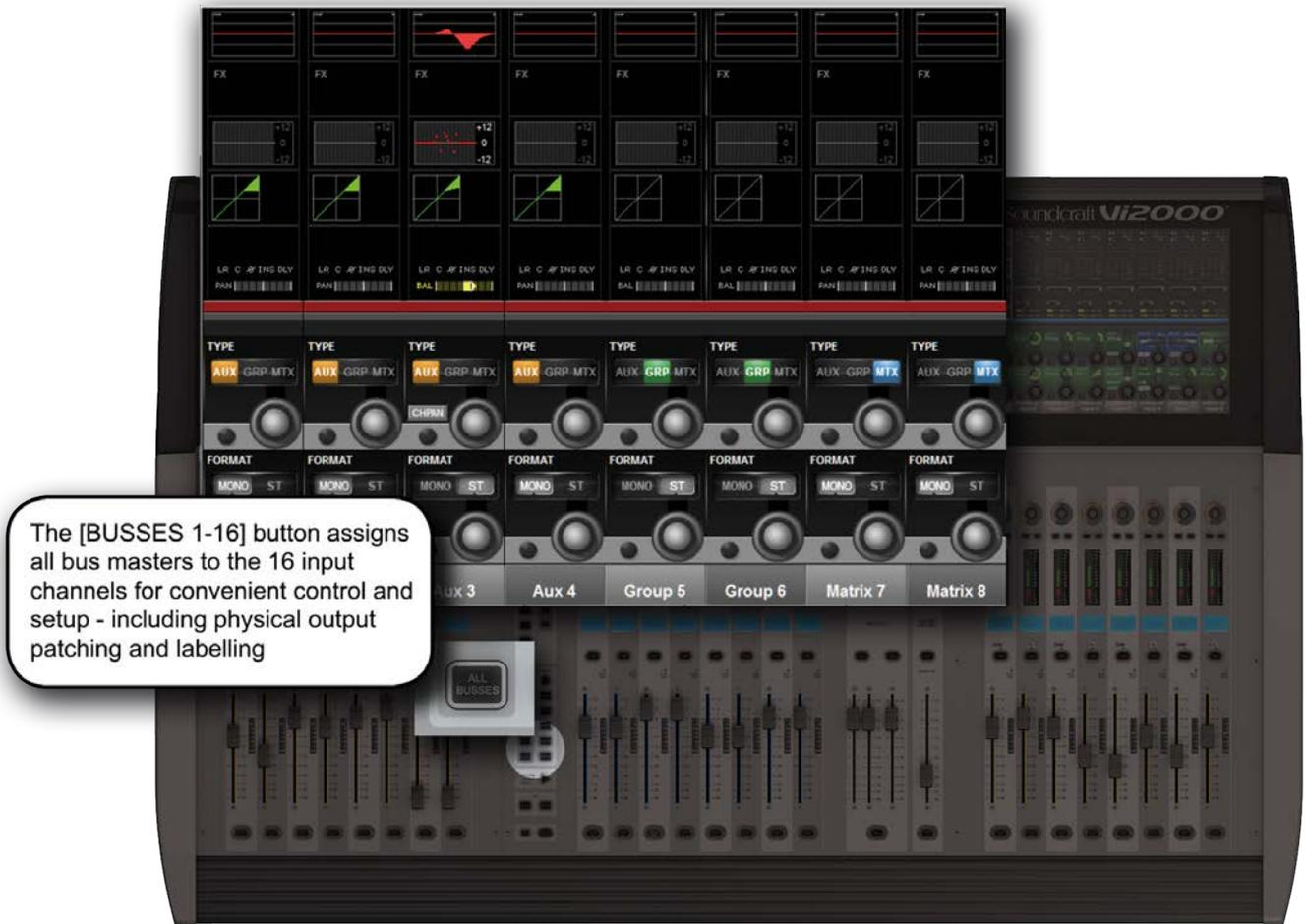
The [BUSES 1-16] button assigns all bus masters to the 16 input channels for convenient control and setup - including physical output patching and labelling
