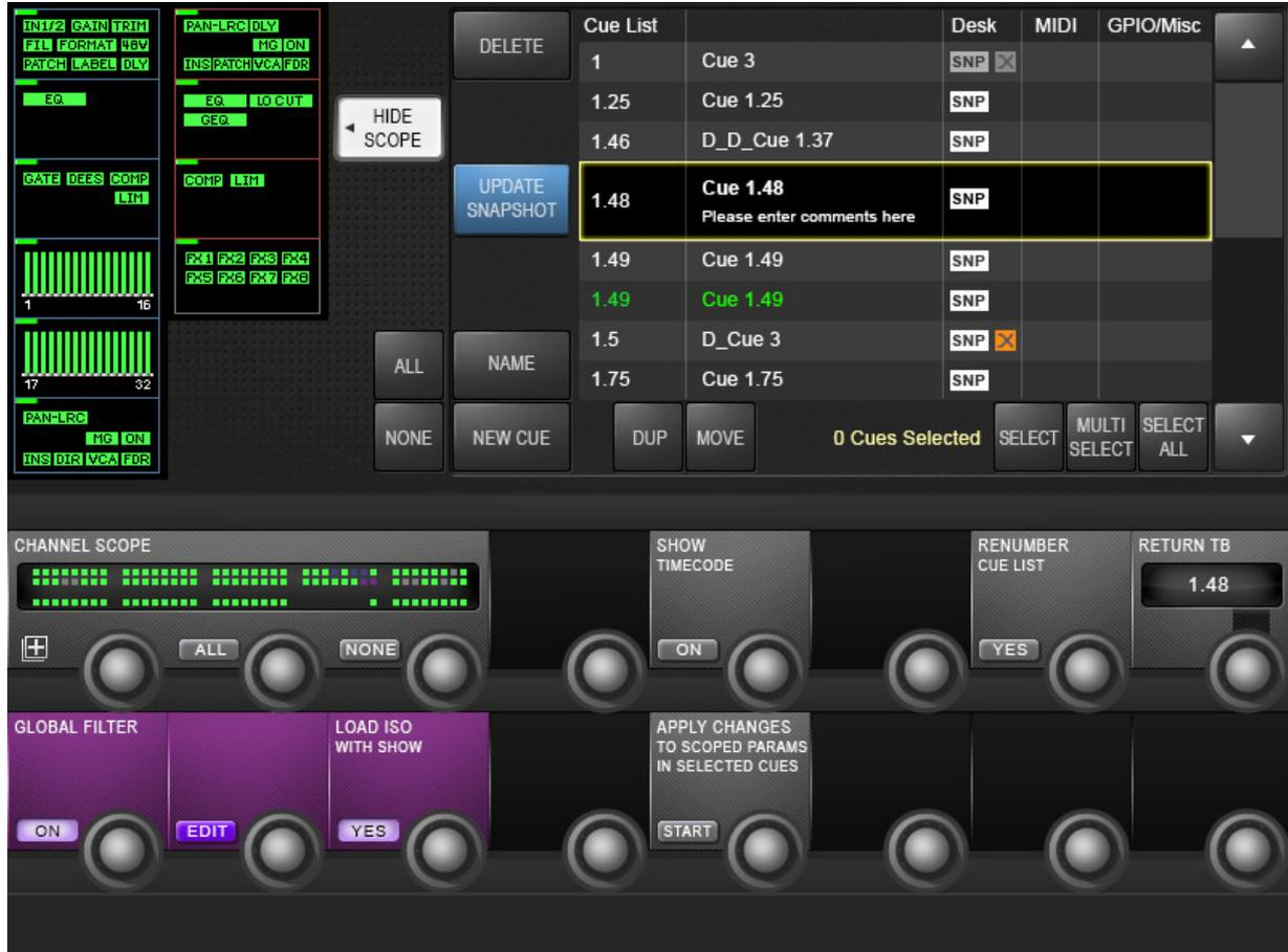
Snapshot filtering is a way of preventing certain settings on the console from changing when a Cue is recalled. There are two different reasons why this is useful, and therefore there are two different types of snapshot filtering: Global Filtering (also called Isolation), and Snapshot Scope.
