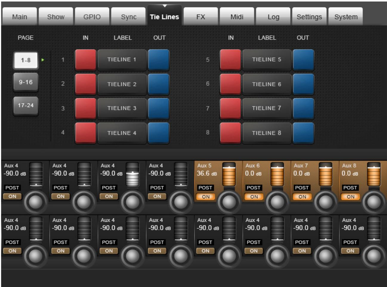
TIE Lines are direct connections from an input connector to a output connector. They are a path through the mixer with no processing and no mixing, and there they do not use up any DSP channels. The console supports up to 24 tie lines, arranged 8 per page.
