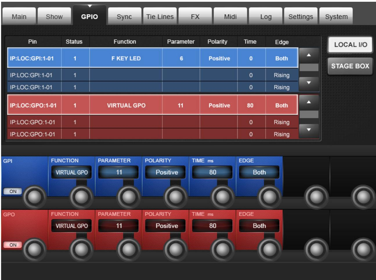
You can configure all available GPIO channels in the GPIO (General Purpose Input Output) tab of the main menu. However, please note that 'virtual' GPIO pins can also be assigned to cues in the cue list via the Snapshot SETUP page. Virtual GPIO Pins are assigned via the function/parameter setting in the main GPIO settings.
