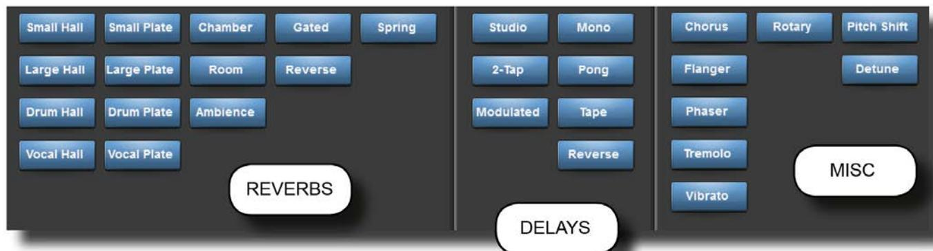
For each of the four FX processors an individual FX Type can be selected. The FX Types are grouped into the following categories: Reverb, Delay, and Miscellaneous. You can select algorithms by hitting the {TYPE} button in the VST section of any FX page.
