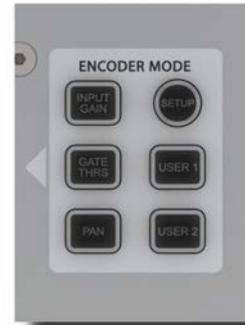
The Input Bay ENCODER MODE group of buttons determines the input channels' encoder 3 function.
