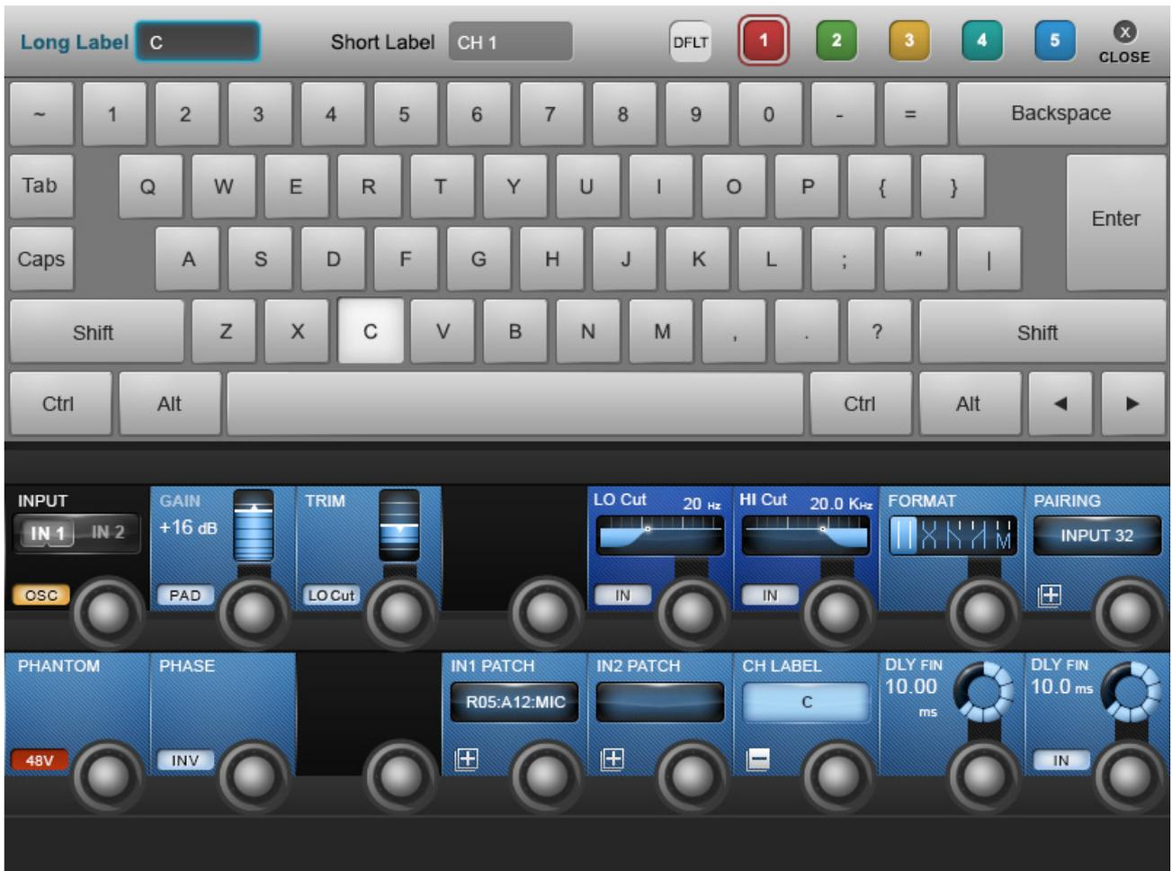
The console labelling system is displayed on a touch-screen area whenever the labelling of a channel, output, cue, file, or other named parameter or item is required. For example, you can label an input channel by touching the channel's input area on the touch screen then pressing the {CH LABEL} button in the VST area.
