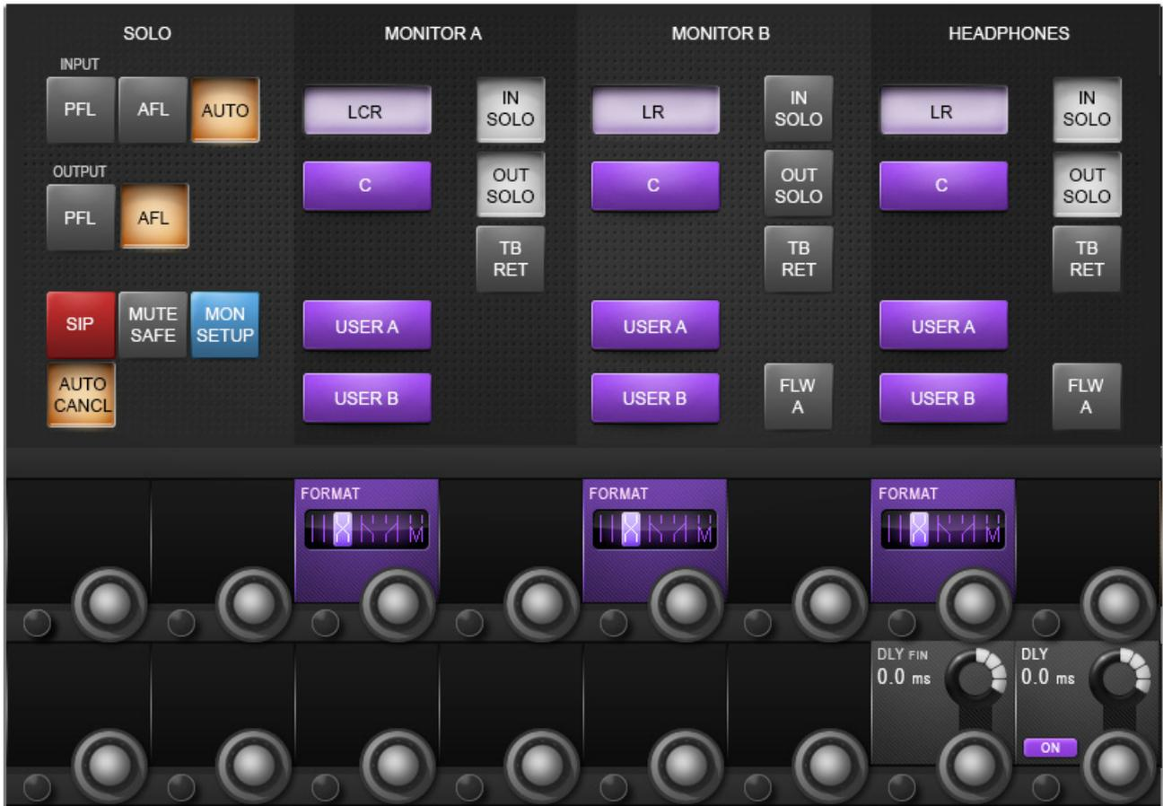
All monitoring source assignments for MONITOR A, B, and HP are assigned in the monitoring setup page, as well as monitoring delay.
