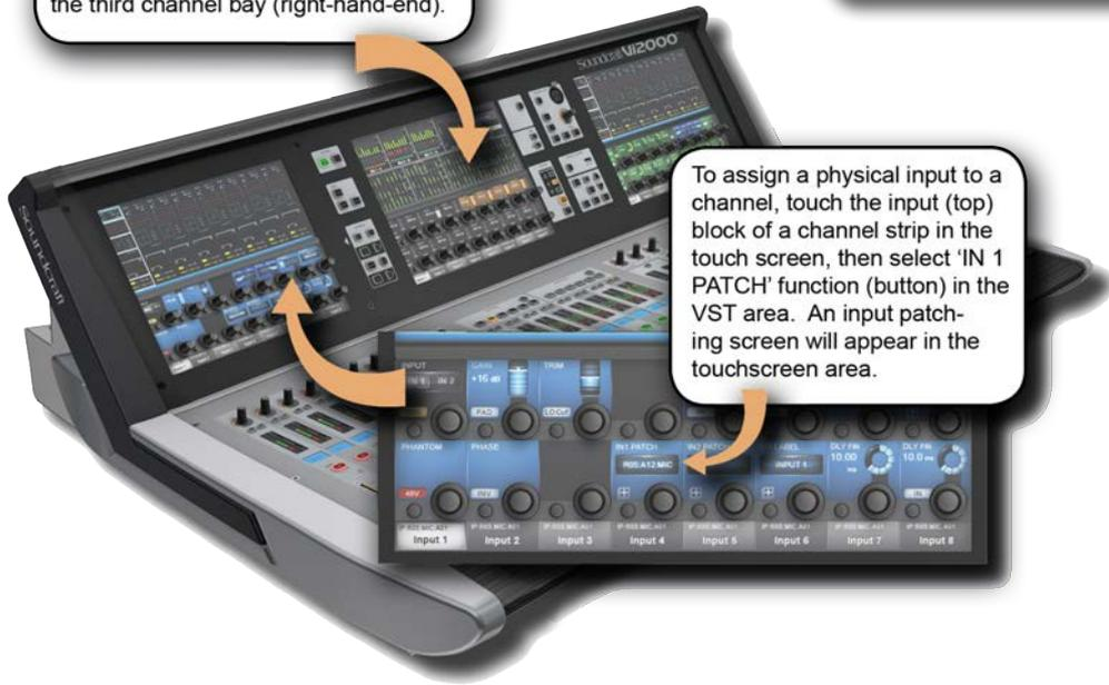
To assign a physical input to a channel, touch the input (top) block of a channel strip in the touch screen, then select 'IN 1 PATCH' function (button) in the VST area. An input patching screen will appear in the touchscreen area.
