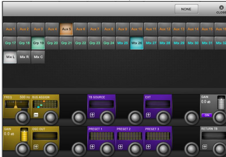
Talkback return allows the console operator to route inputs directly into the monitor circuit. This allows assistants within a venue to talk directly to the console operator. The talkback function must be enabled via the MONITORING setup page by selecting the TB RET touchscreen button for Monitor A, B or Phones outputs.
