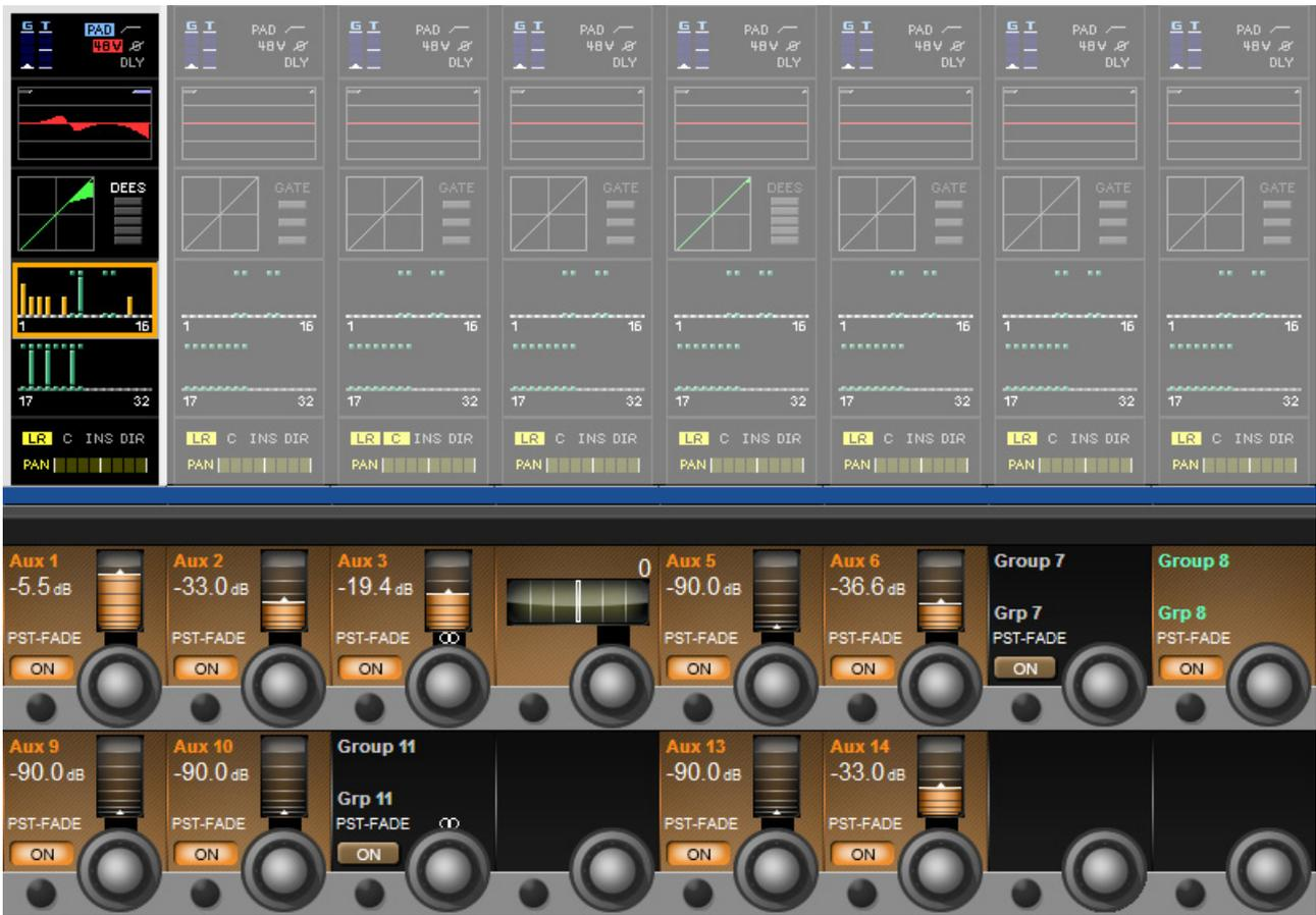
The Busses section of the input channel vistonics touch screen signal path provides access to all Aux and Group contributions in the VST area. The Touch Screen block graphic shows activated Aux levels in orange and group routings in Green. The controls vary depending on whether you are working on Auxiliaries or groups.
