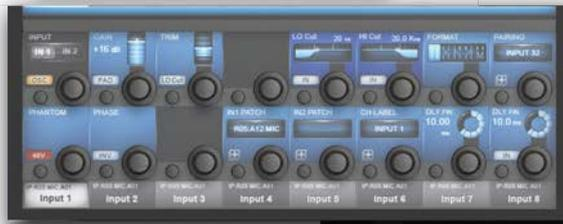
The Input Bay VISTONICS buttons allow convenient, rapid access to output contributions on the Input Bay Vistonics encoders.
