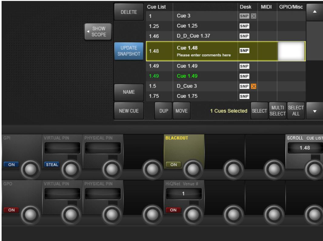
Selecting a the GPIO column in the cue list gives access to that cue’s GPIO (General Purpose Input Output) settings. The VST screen is split into GPI (input) and GPO (output) sections. The inputs section sets an input to be used as a recall trigger for this cue, while the output section defines an output to be triggered when the cue is recalled. The cue GPIO system uses ‘virtual pins’ that are mapped to physical pins in the master GPIO settings screen.
