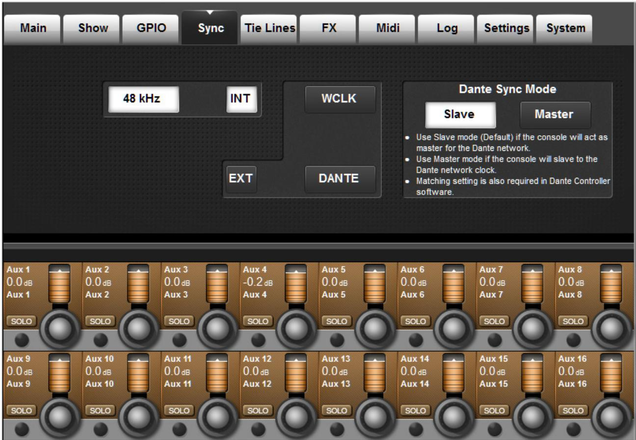
The settings in this tab determine the digital audio clock configuration for the console
