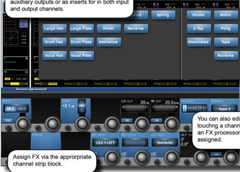
Assign FX via the appropriate channel strip block.
