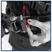
If the rig tends to move straight **away** from you; loosen the bottom thumbscrew and slowly tighten the top thumbscrew until the rig is neutral.
