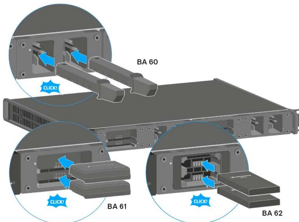
**i** At ambient temperatures of 45° C (113° F) and above, the rechargeable batteries can no longer be fully charged. They can only be charged to a maximum of 70 %.
