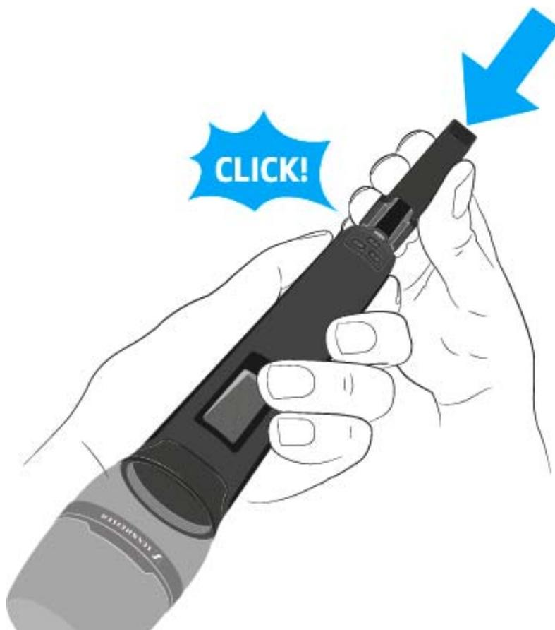
To remove the B 60 battery compartment from the SKM 6000 handheld transmitter:
