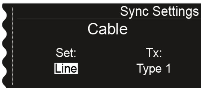
The **Cable** function is a cable emulator that you can in 3 stages (**Type 1**, **Type 2**, and **Type 3**). Cable emulation is switched off with the **Line** option.
