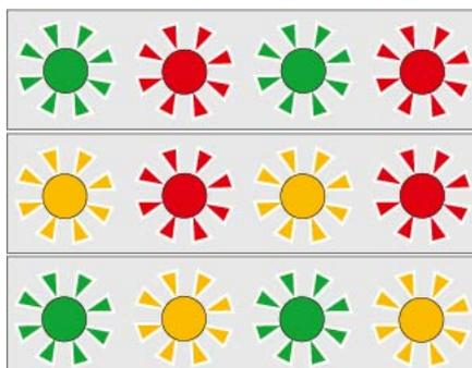
**Flashing green/red** >> rechargeable battery not inserted.
