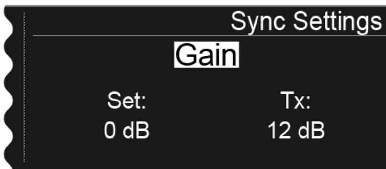
The top line displays the option that is currently selected (Gain, Low Cut, Auto Lock, Display, Cable).
