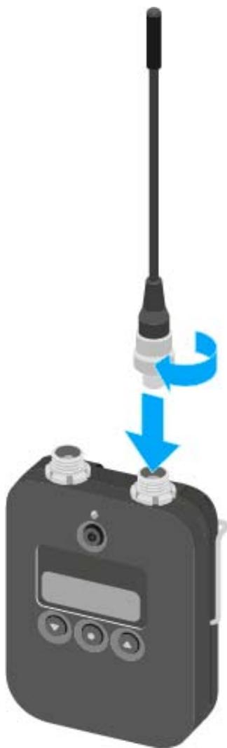
**i** The antenna can be connected to the antenna socket very gently in only one direction. Do not use force to connect the antenna to the bodypack transmitter antenna socket.
