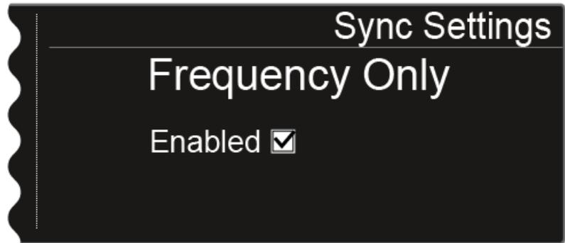
If this option is activated, only the frequency is transmitted to the transmitter. No other options are transmitted, regardless of their settings.
