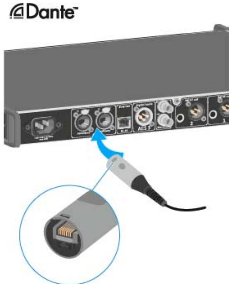
We recommend using an Ethernet connector as shown in the figure.
