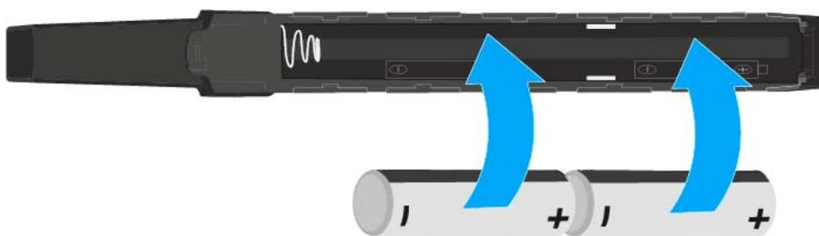
To insert the B 60 battery compartment into the SKM 6000 handheld transmitter:
