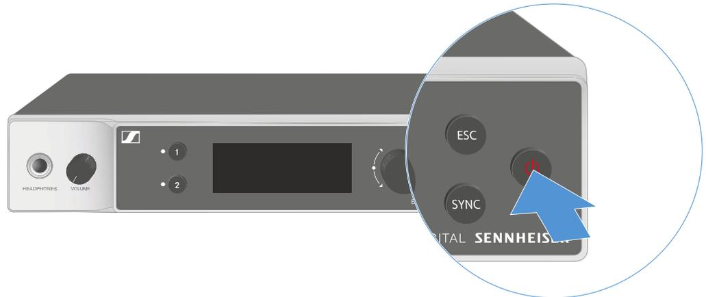
To switch the receiver to **standby mode**:
