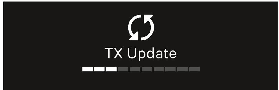
The transmitter's display shows that the firmware update is in progress.
