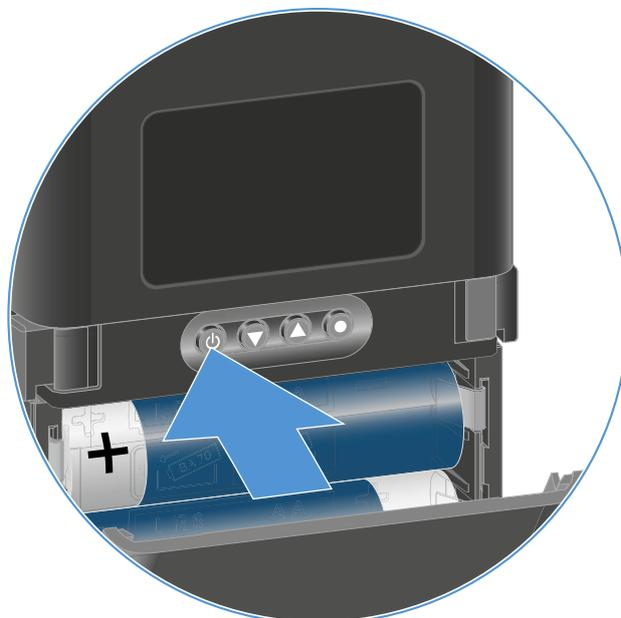
To switch the bodypack transmitter off:
