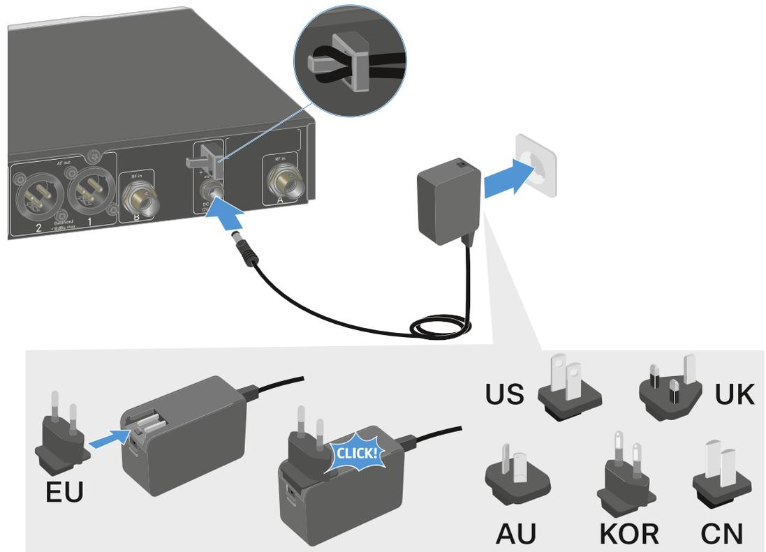
To completely disconnect the receiver from the power supply system:
