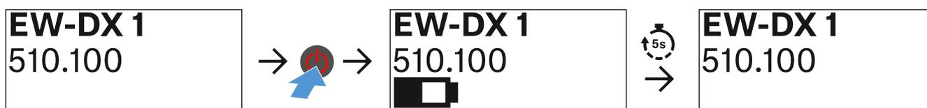
Pressing the transmitter's **ON/OFF** button will simultaneously trigger the Identify function: "Identifying the paired receiver (Identify function)".
