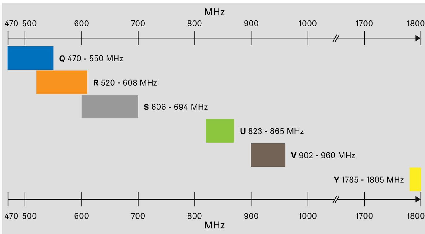
The **EW-D ASA** antenna splitter is available in the following frequency ranges:
