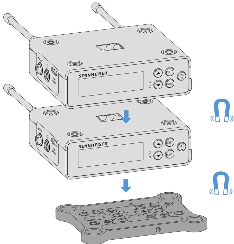
The receiver has magnets on the bottom, which means you can simply place it on the mounting plate without the need for an additional screw connection. This allows you to stack two receivers on top of one another.
