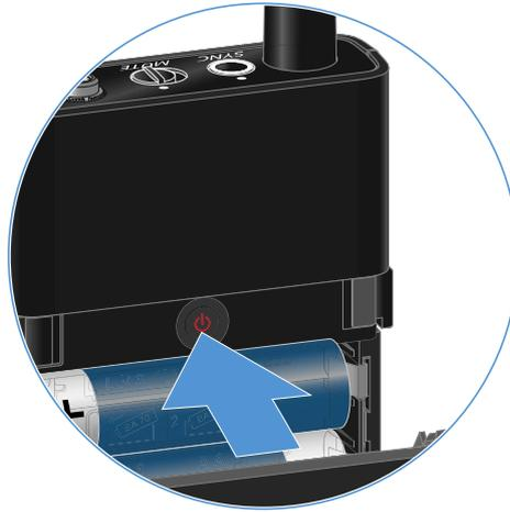
To switch the bodypack transmitter off:
