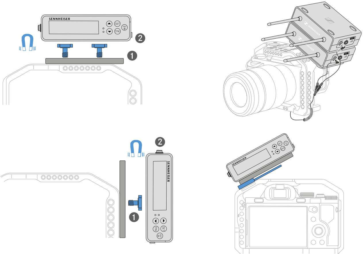
To attach the mounting plate to a **camera cage**:
