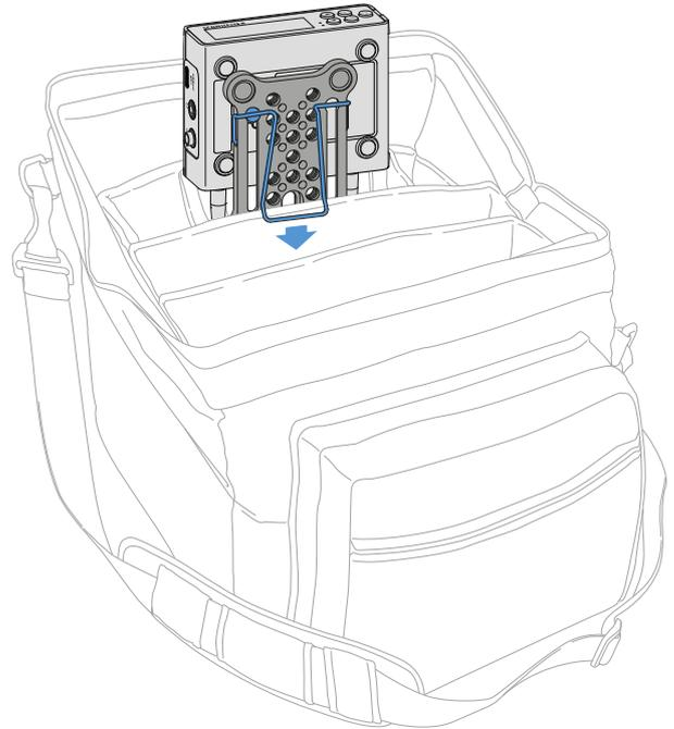
To fasten the receiver with mounting plate to **pockets or belts**:
