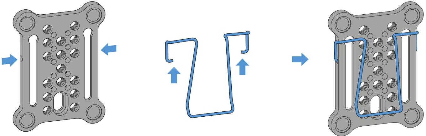
As an alternative to the hot shoe adapter, a **metal clip** can be attached to the side of the mounting plate.
