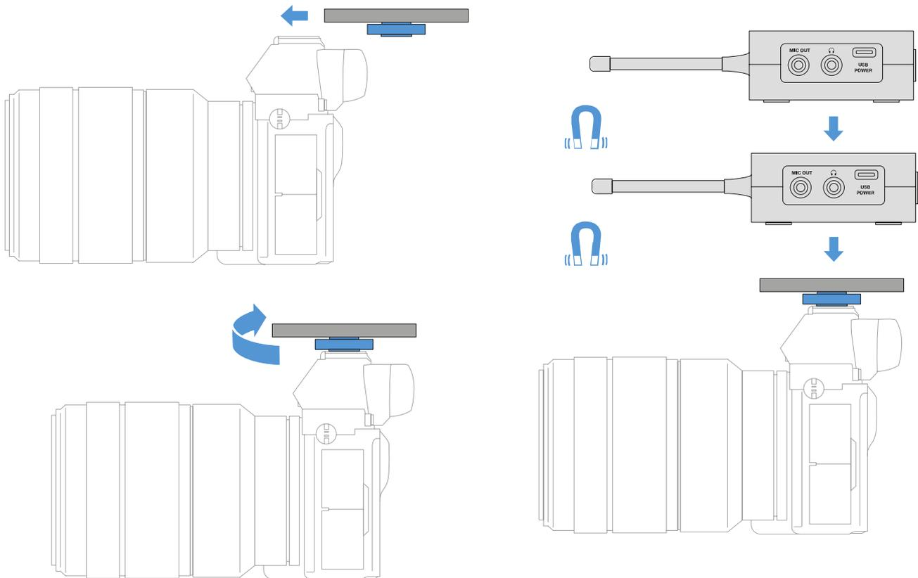
To mount the mounting plate with hot shoe adapter on a **DSLR or video camera**:
