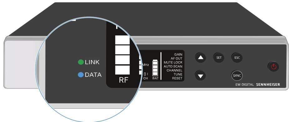
The **LINK** and **DATA** LEDs on the front of the receiver can indicate the following information.
