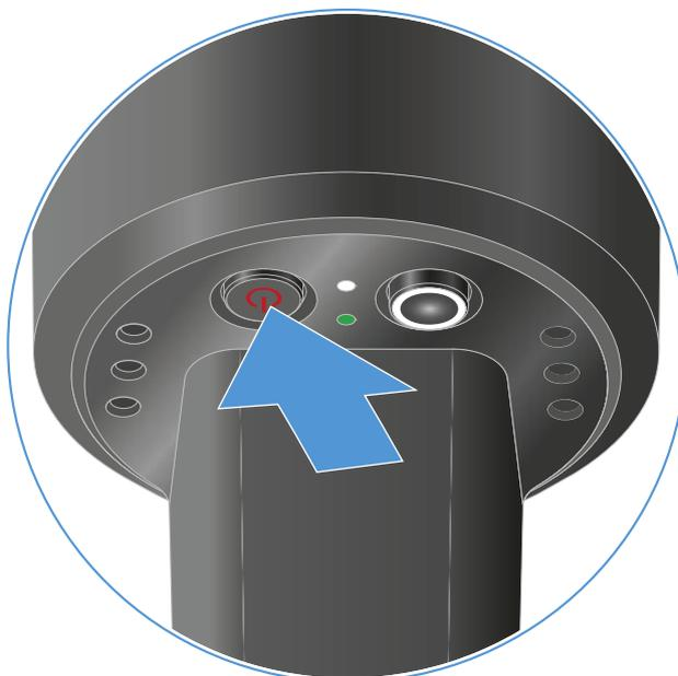
To switch the handheld transmitter off:
