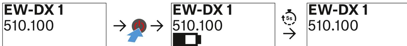
Pressing the transmitter's **ON/OFF** button will simultaneously trigger the Identify function: "Identifying the paired receiver (Identify function)".
