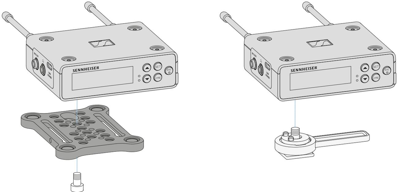
To mount the receiver with the mounting plate rotated by 90°:
