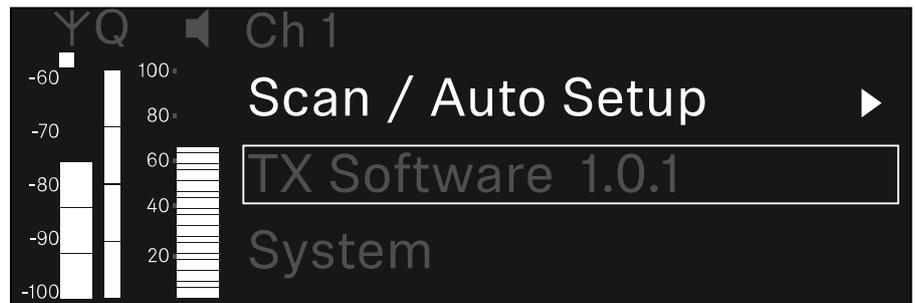
The version number of the transmitter software is shown on the display.
