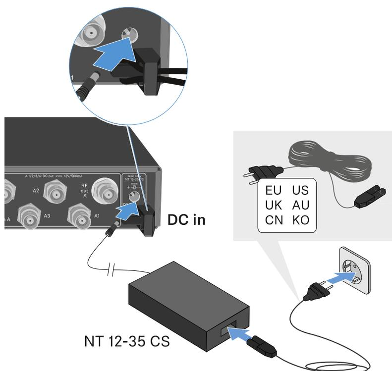
To completely disconnect the EW-D ASA antenna splitter from the power supply system:
