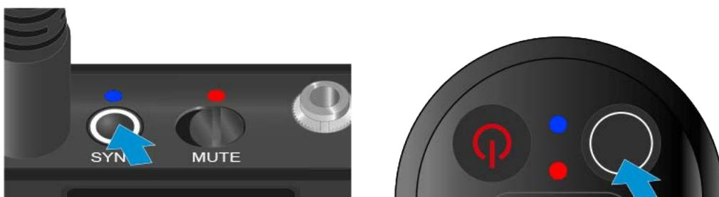
The transmitter and receiver will be paired. Once the link is established, the **LINK** LED on both units will light up green.
