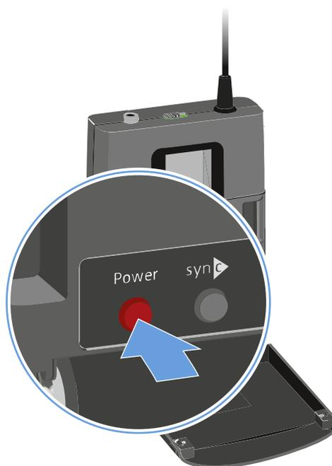
To switch the bodypack transmitter off:
