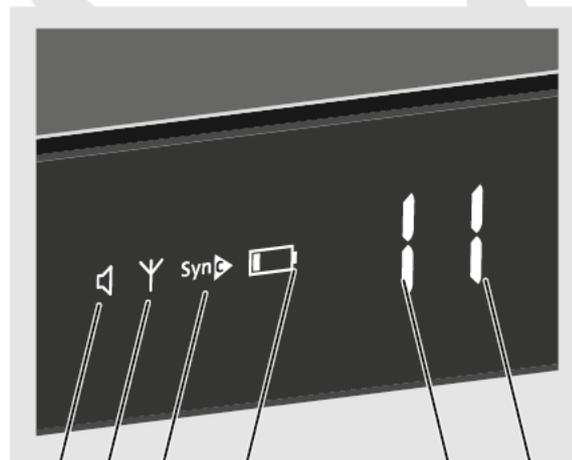
Sensitivity RF Sync Battery Bank 1 - 8 Channel 0 - 9
