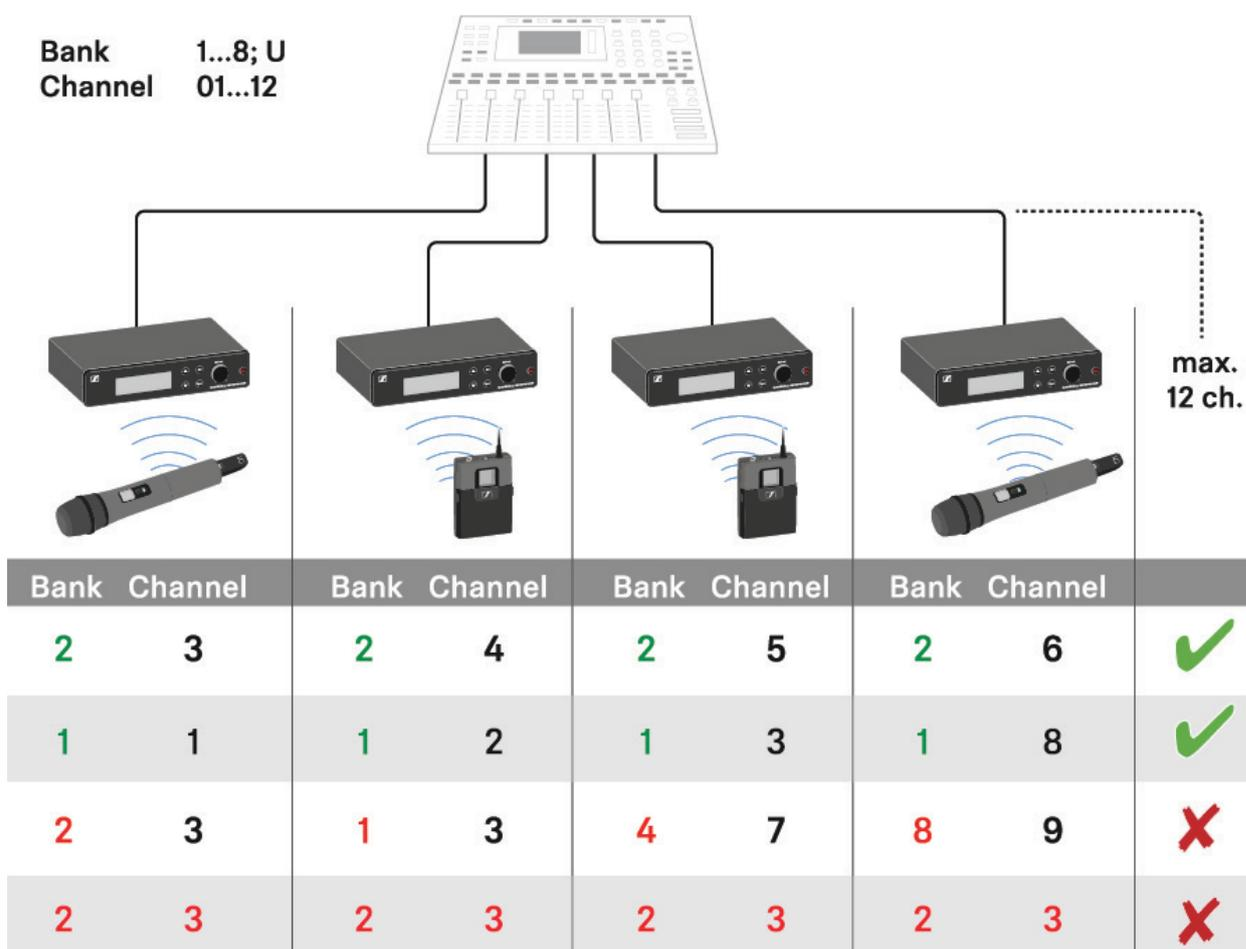
We recommend using the **SCAN** function, as this is the most reliable way to identify free frequencies (see „SCAN menu item“).
