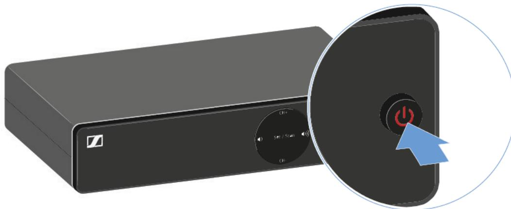
To switch the receiver to **standby mode**:
