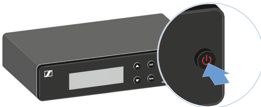
To switch the receiver to **standby mode**:
