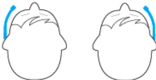
The neckband has a total of five clips which are designed so that the microphone boom can be worn on either side of the mouth.
