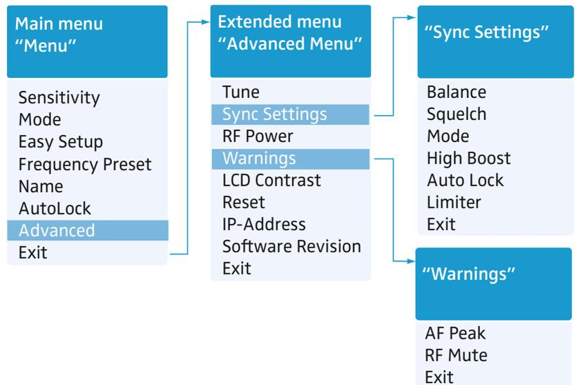
When the standard display is shown on the display panel, you can get into the main menu by pressing the jog dial. The extended menu **"Advanced Menu"** and the other menus can be accessed via the corresponding menu items.
