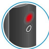
The charge level of the **connected** transmitter/receiver is below 15%.
