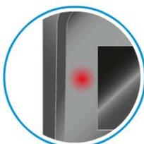
The charge level of the **connected** transmitter is below 15 %.
