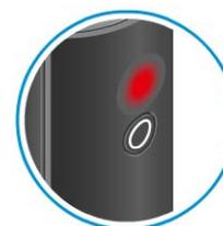
The charge level of the **connected** transmitter/receiver is below 5%.
