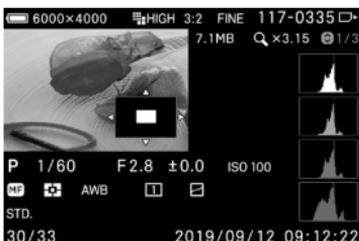
To enlarge an image and view the detailed histogram in a specific area, rotate the Front dial clockwise or pinch out on the touch panel while image information is being displayed.
