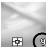
The number in the bottom right of the LCD monitor indicates how much buffer is left. It is the maximum number of frames for continuous shooting. (If the maximum number of frames for continuous shooting exceeds nine frames, the display will not change from **9**) When the number becomes "0", the shutter cannot be released.
