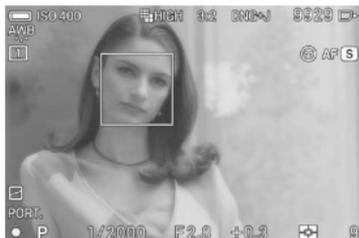
When a face and an eye are detected, the orange detection frame is displayed. When the detected face and eye are focused after the shutter button is half-pressed, the detection frame changes to green.
