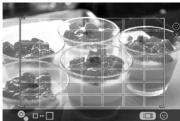
The range of the distance measurement area can be changed by pressing the **AEL** button and turning the Front/Rear dial (the size of the multi-point distance measurement area frame is changed).
