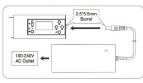
When a supplied AC power supply is connected to the fixture, it will provide power for the fixture to operate and/or charge the rechargeable battery pack depending if the battery is inside or not.
