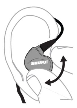
Note: Do not pull on cable to remove earphone.
