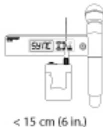
4. sync good appears on the display when IR sync is complete. The blue rf LED will illuminate indicating that the transmitter is within range of the receiver.
