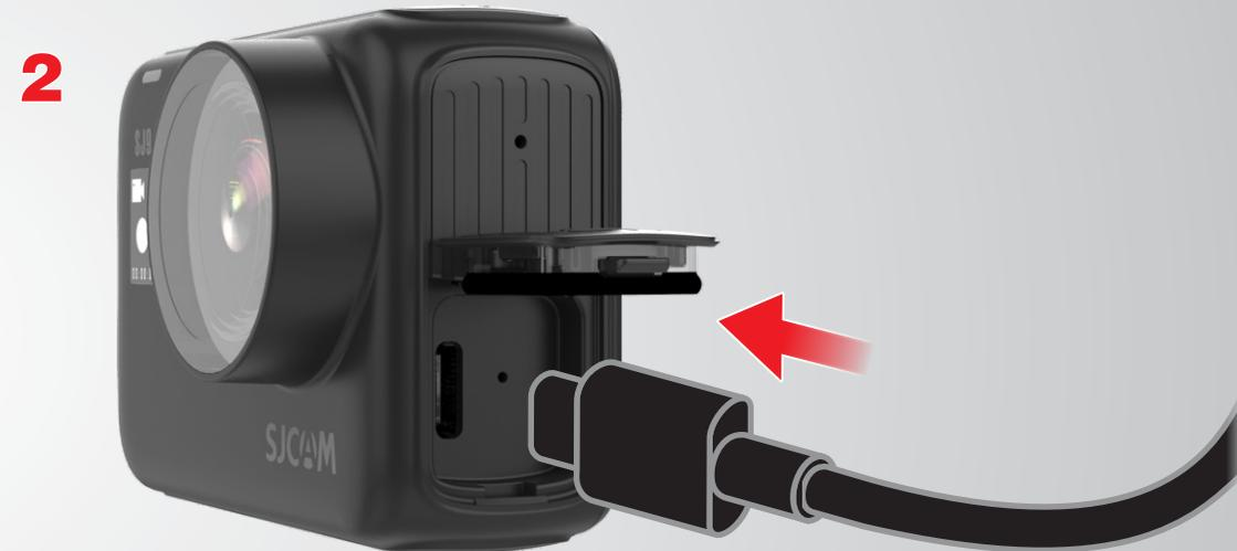
Locate the covered USB-C port on the left side of the camera. Use a fingernail to slide the lock open. Swing the door outwards.
