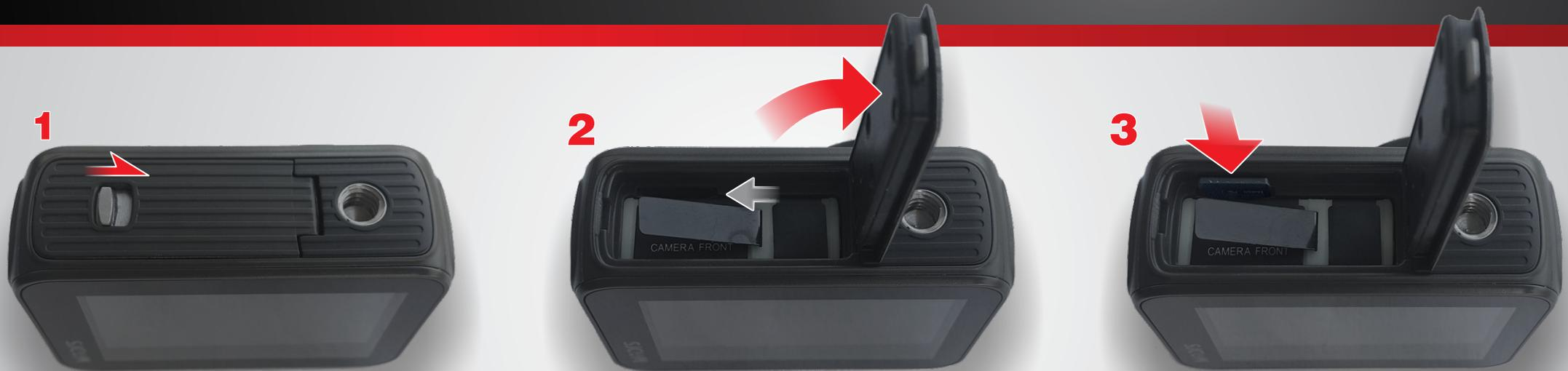
Open the battery cover by sliding the lock with your fingernail towards the direction shown above.
