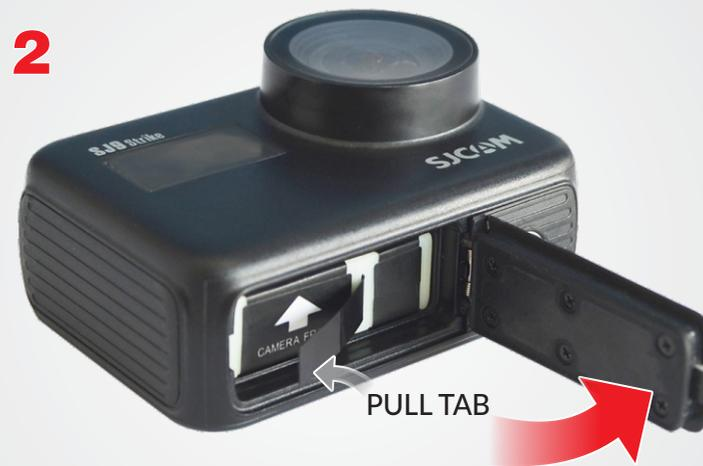
2 While pressing on the lock, swing the battery door open. Grab the pull-tab with your fingers.
