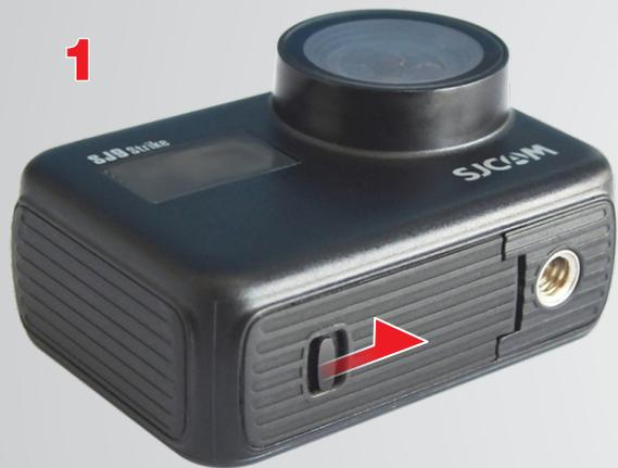
1 Open the battery cover by sliding the lock with a fingernail.
