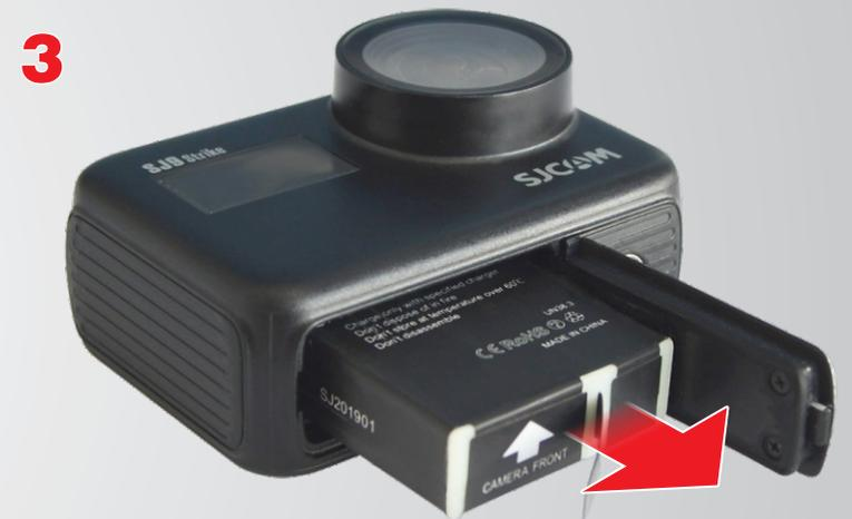
3 Pull the battery out. Insert a freshly-charged battery in.
