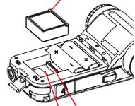
Transmitter Module Compartment **18**
