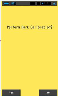
**2. Turn the Light Selection Ring ② to set to the dark calibration position CAL (
