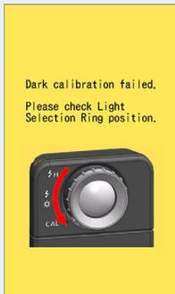
While the dark calibration is being performed, the position of Light Selection Ring ② is changed. so dark calibration could not be completed normally. Set the Light Selection Ring ② to the dark calibration position **CAL** (🔌) again, and perform dark calibration again.
