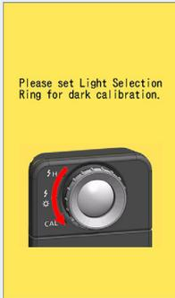
The Light Selection Ring ② is set to Range H (⚡) or Range L (⚡), and dark calibration could not be performed.
