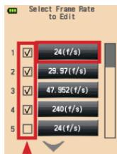
Check to display or not in the Frame Rate setting in the Measuring Screen
