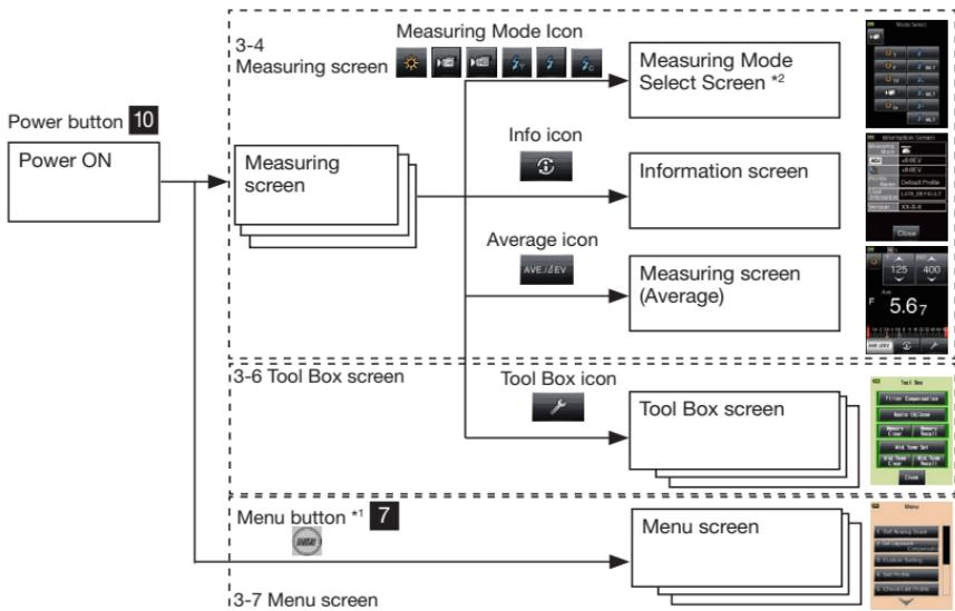
\*1 If you press the Menu button while working at another Setting screen, the settings in mid-operation will be interrupted and the Menu List displayed.
