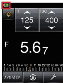
When the power is turned on, the battery power indicator is displayed at the upper left of the LCD.
