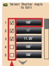
Check to display or not in the Shutter angle setting in the Measuring Screen
